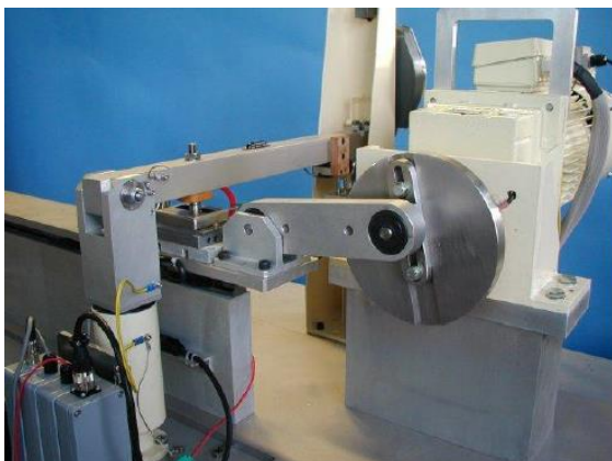
Figure 24: TE 88 test machine configured in pin on plate mode [39]
