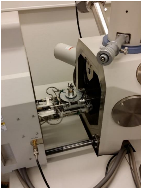
Figure 28: The samples mounted in the energy dispersive x-ray spectroscopy (EDS)
