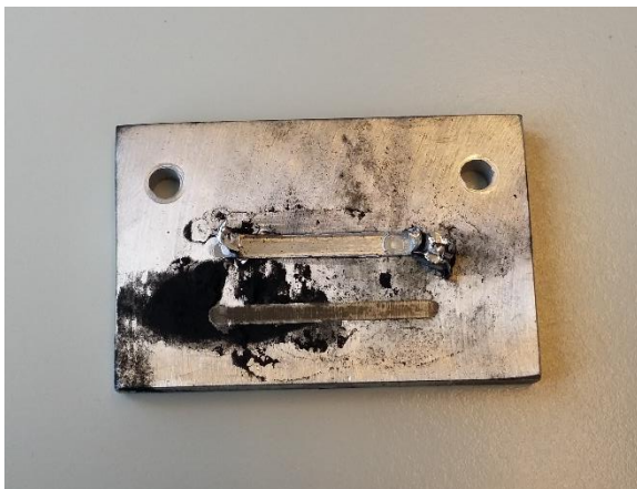
Figure 29: The wear track on top is where the lubricant failed, and the wear track on the bottom is when the lubricant worked successfully
