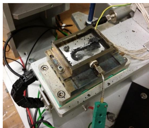
Figure 25: The plate with solidified Lubrodal F 33 Al, after the test
