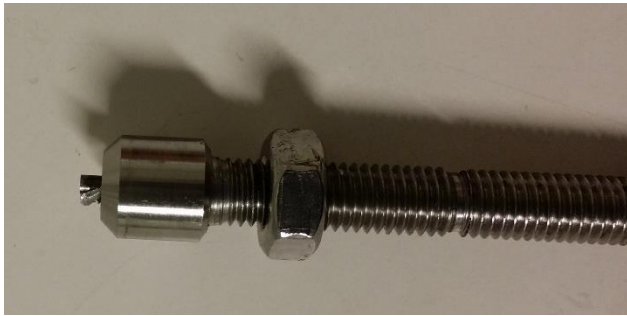
Figure 40: Pin in pin-holder, with aluminium sticking to the pin
