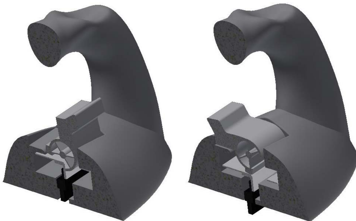
Figure 14-7: Half section view of model with brush in up position (left model) and down position (right model)
