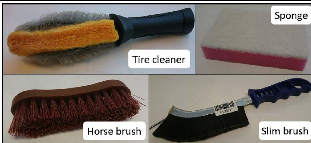
Figure 7-6: Some of the brushes used in dirt cleaning experiment
