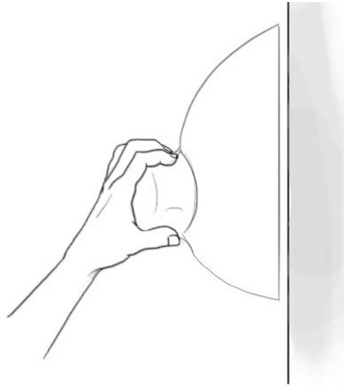
Figure 13-9: Round “joystick” handle
