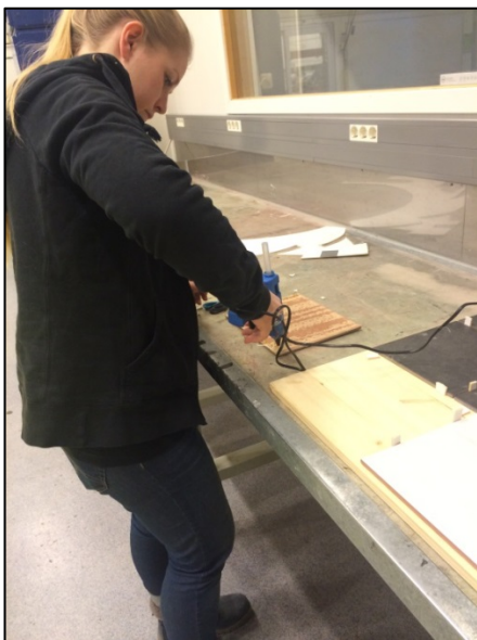
Figure 7-2: Adding glue to the tile and placing it to the wood board
