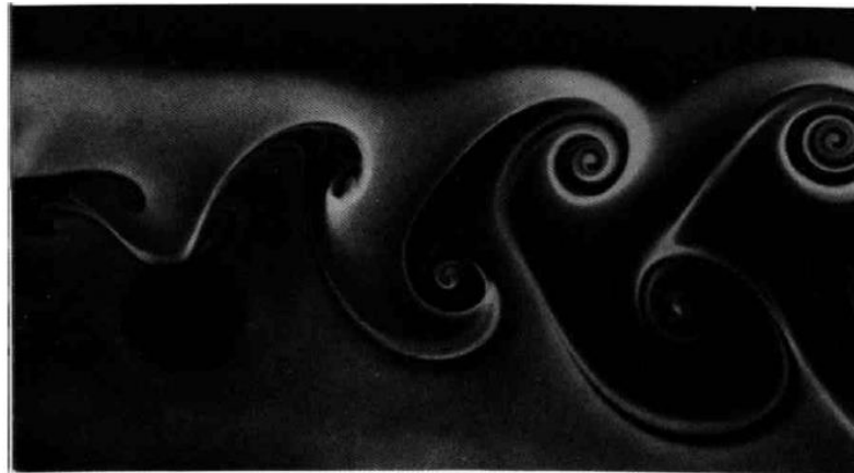
Figure 3.4 Karman vortex sheet behind the cylinder for Re=200 . Photograph by Gary Koopman [4]
