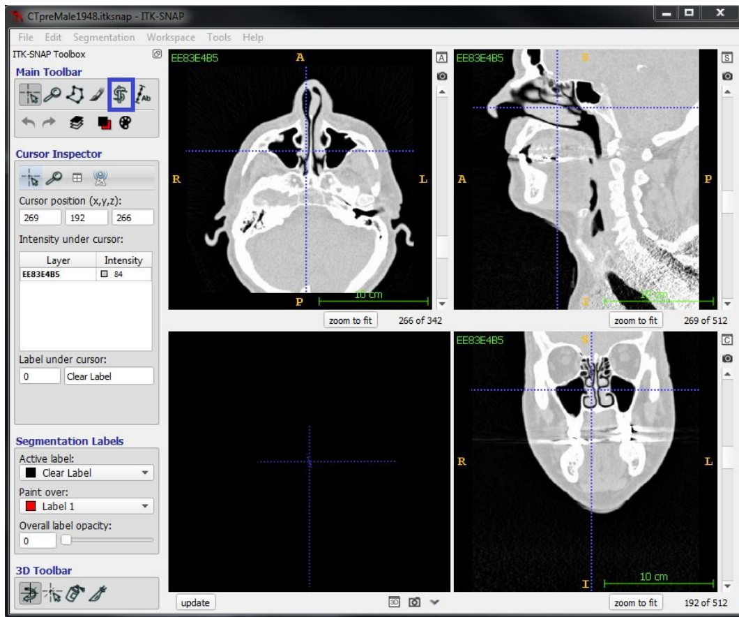
Figure 7: The DICOM files as they appear in ITK-SNAP 3.4.0. Active Contour Segmentation is marked with a blue square.
