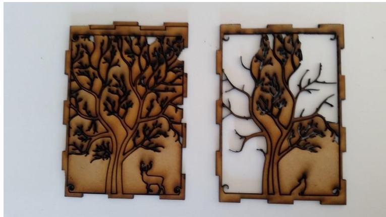
Figure 13: Fine cut burned vs unburned
