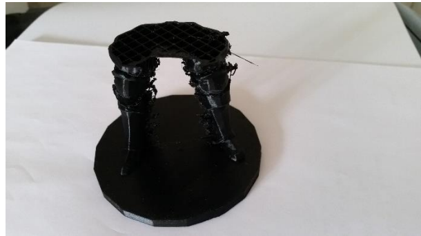
Figure 15: Aborted knight print, no shield
