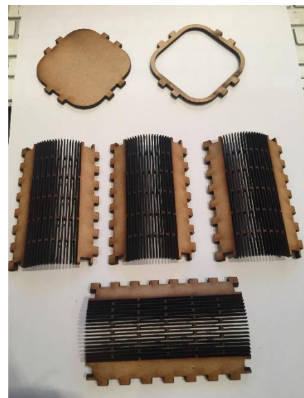
Figure 11: Living hinge pencil holder parts
