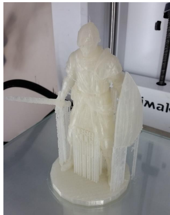
Figure 16: Knight, with support structure under the sword and shield, between the legs and under the arms
