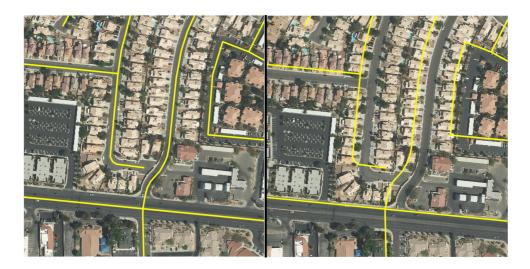
Figure 6.13: UrtheCast: Comparison of good and poor absolute geolocation accuracy. Credit: UrtheCast [Urtc].
