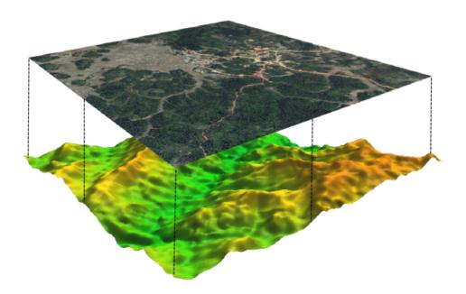
Figure 3.1: Multispectral image being projected on a DEM. Credit: Sylla Consult [Syl].
