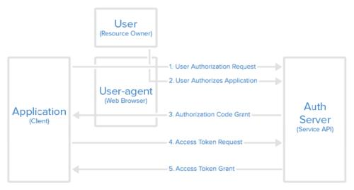
**Figure 3.10:** OAuth2's protocol flow when working with server-side applications. Credit: DigitalOcean [Ani14].
