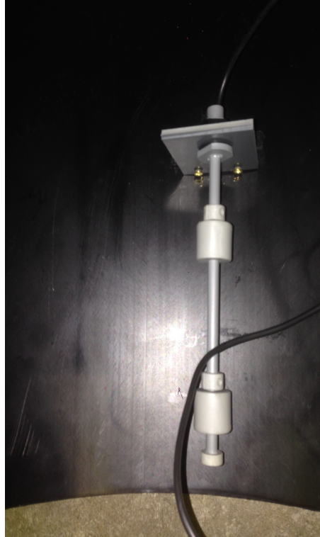
Figure 3.8: Level transmitter mounted in the separator. The picture was obtained when the separator was upside down. Therefore the floaters are in the upper position.
