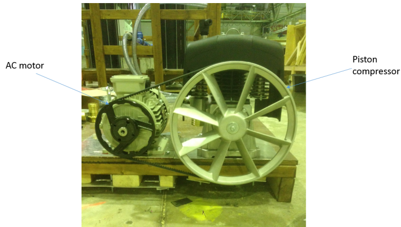
Figure 3.14: Belt driven piston compressor with electrical motor.
