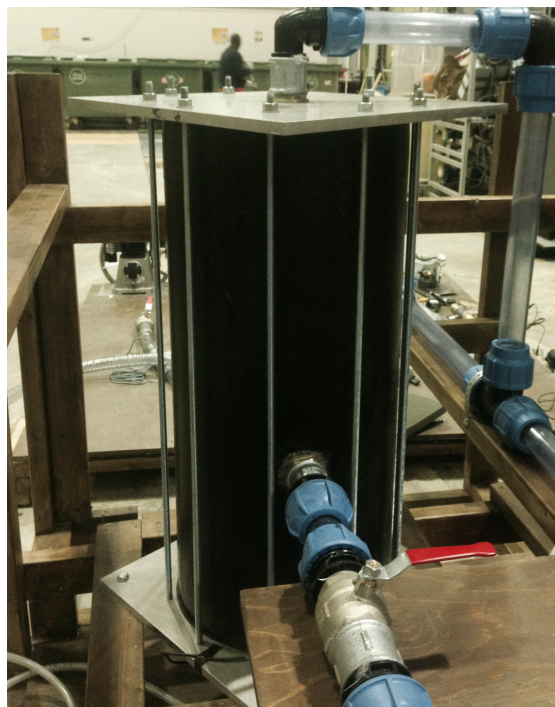
Figure 3.3: The separator mounted in the frame.
