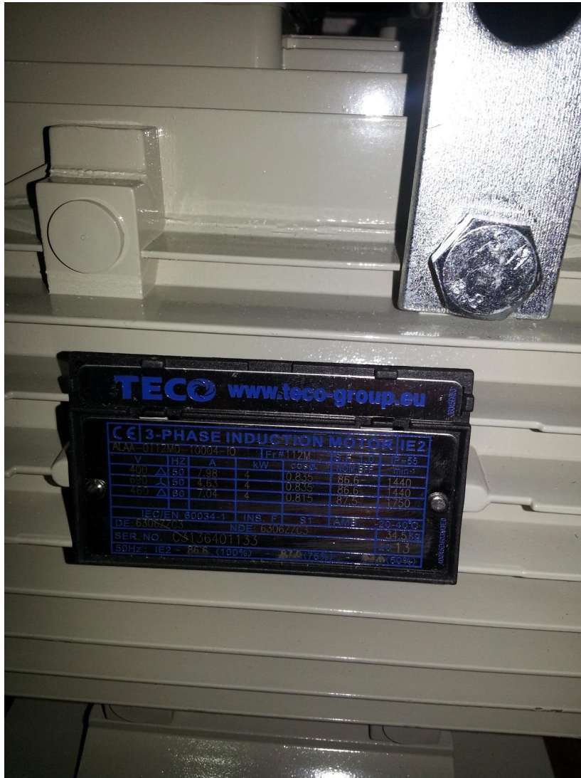
Nameplate for 4000kW induction motor for piston compressor
