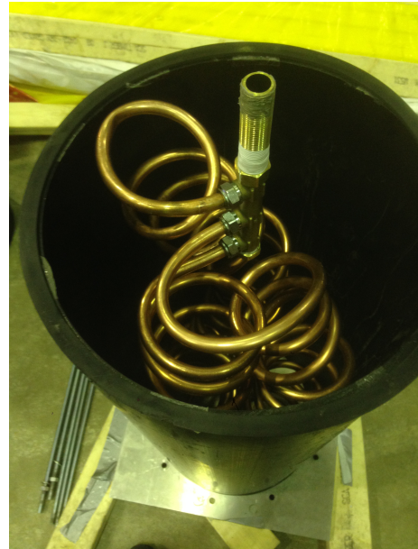
Figure 3.12: Copper helix inside the cooler shell.
