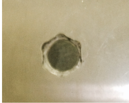
Figure 3.13: The milled hexagonal shape in the aluminium lid
