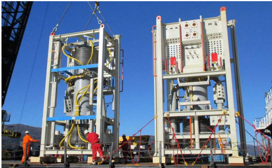
Figure 1.5: The two wet gas compressors installed at Gullfaks [40].
