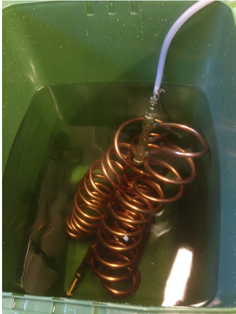
Figure 3.11: The final pressure test of the copper helix.
