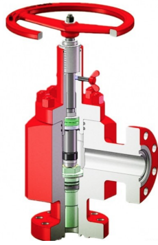
Figure 2.13: Typical design of a choke valve [33].
