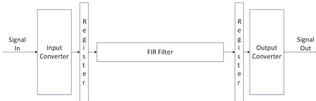
Figure 4.2: Setup of RNS FIR filter simulation
