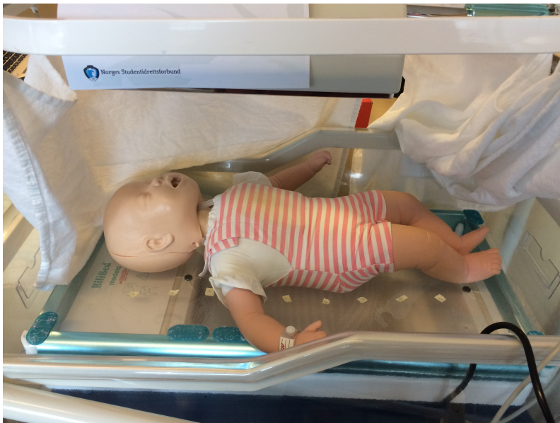
Figure 3.4: Depiction of an infant during phototherapy, approximated with the Baby Anne. The measurement points can be seen on the BiliBed beneath the infant, and covers the area of the baby. Photo taken by the author at the 15 th of March 2016.
