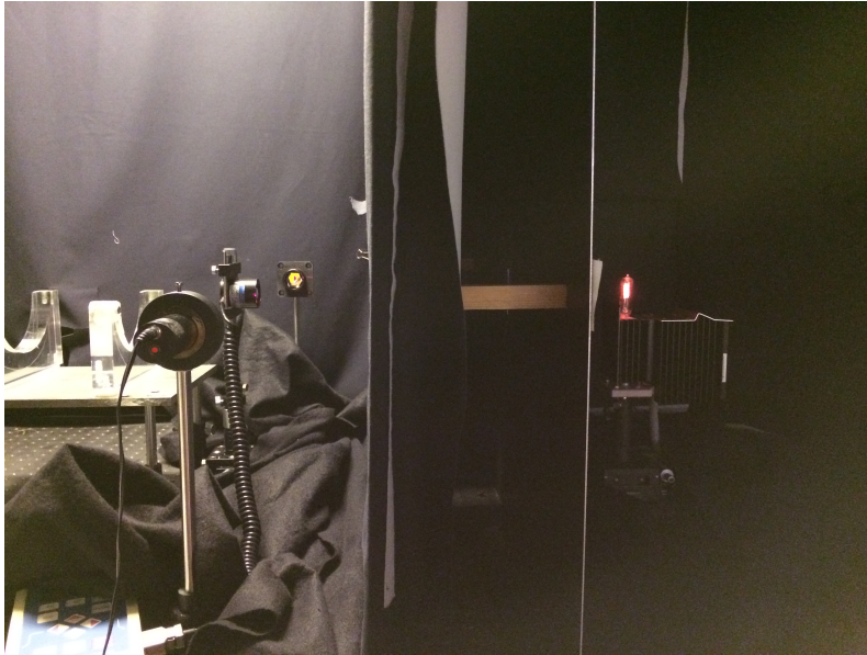
Figure 3.5: The set-up of the calibration of the Blue light safety detector probe with the radiometer. The radiation source was situated on the right side of a black partition with an opening, which directed the radiation directly at the center of the probe. The probe was placed 500 mm from the radiation source. All distances and planes were measured with lasers.
