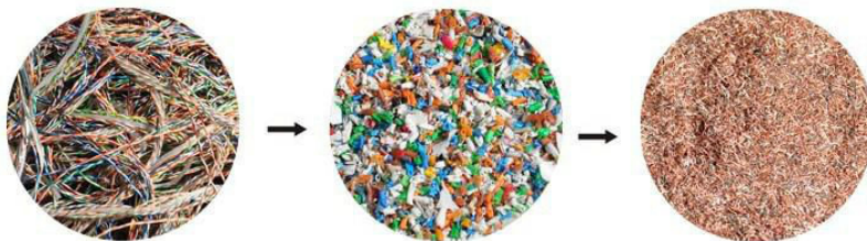
Figure 24 Cable separation process(20)
