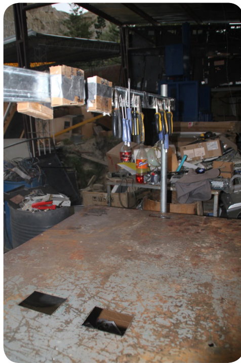
Figure 50 Tool rack with magnets on second prototype
