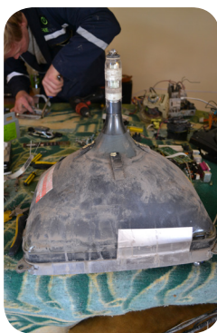
Figure 20 CRT element after stage 1 dismantling
