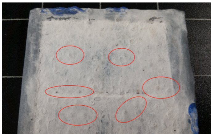
Figure 4.1: Blistering near the scribe on the high Zn primer DFT 50 \mu\text{m} . The picture is taken after 20 cycles of exposure.
