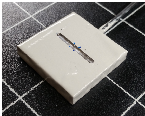
Figure 3.4: Sample geometry of the TSA coated with epoxy. Silicone around the steel wire connection was not yet applied, and is therefore not present in the figure.
