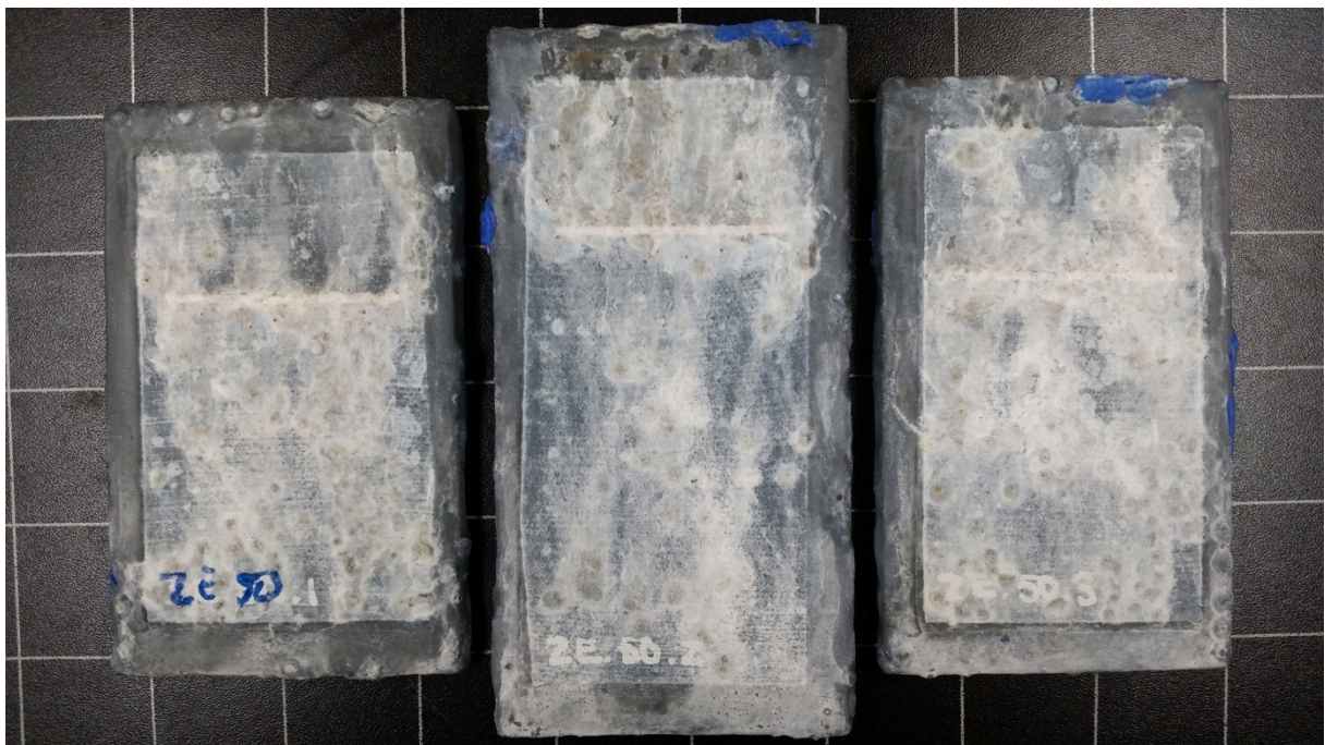
Figure B.4: Visual appearance of the Zn epoxy with DFT 50 \mu m after 20 cycles of exposure.
