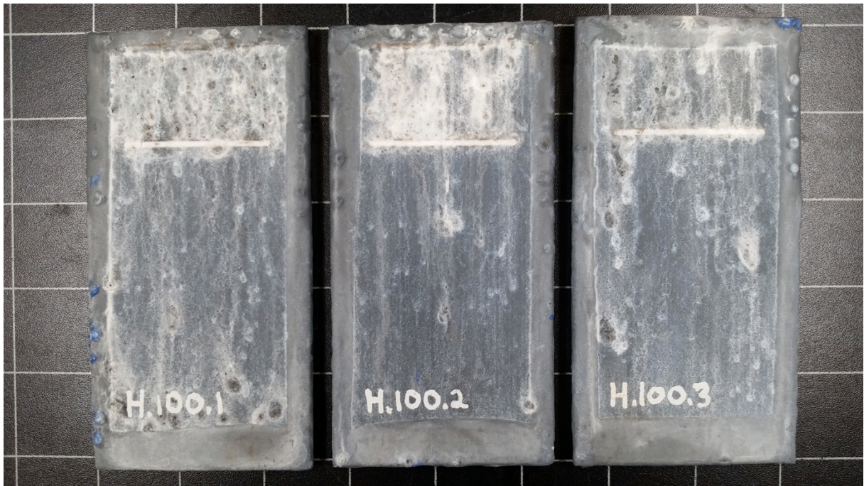
Figure B.11: Visual appearance of the modified Zn epoxy with DFT 100 \mu\text{m} after 20 cycles of exposure.
