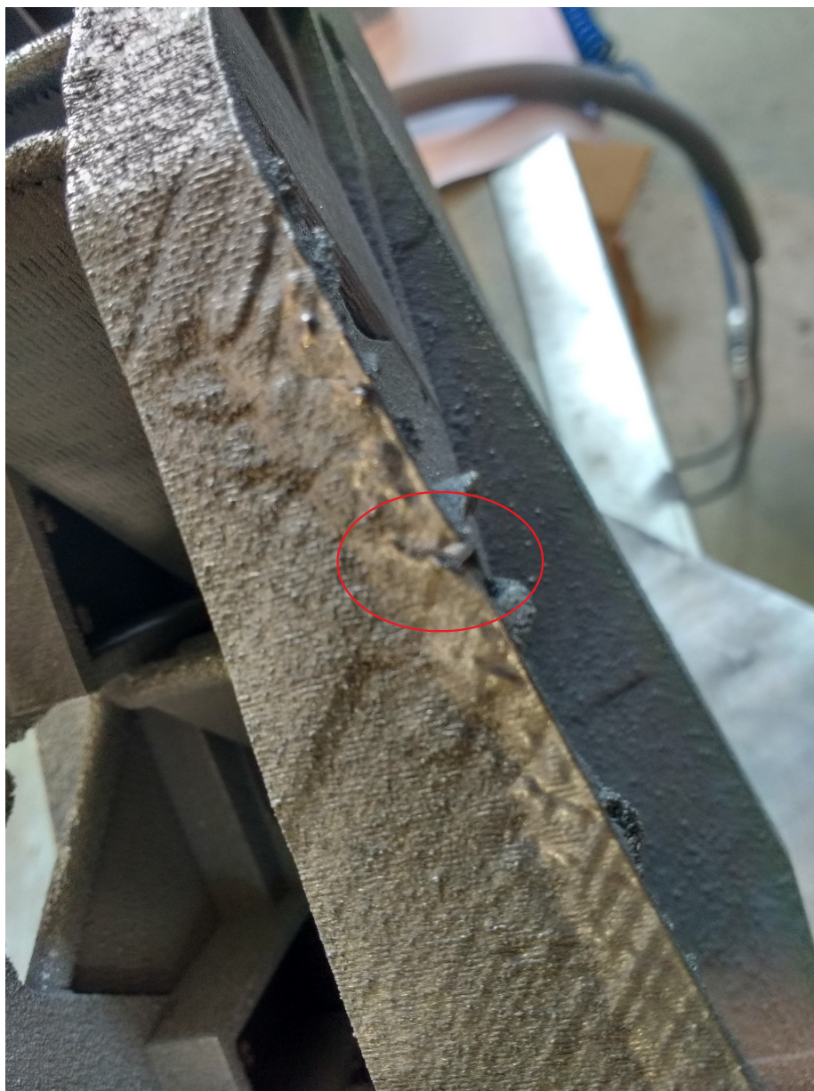
Figure 4.8: Surface roughness and a crack. (circled)
