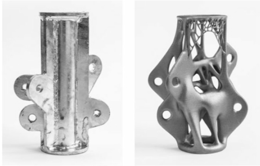
Figure 1.3: A connection node that have been optimized with topology optimization software and built using additive manufacturing.(Source: www.insidemetaladditivemanufacturing.com )
