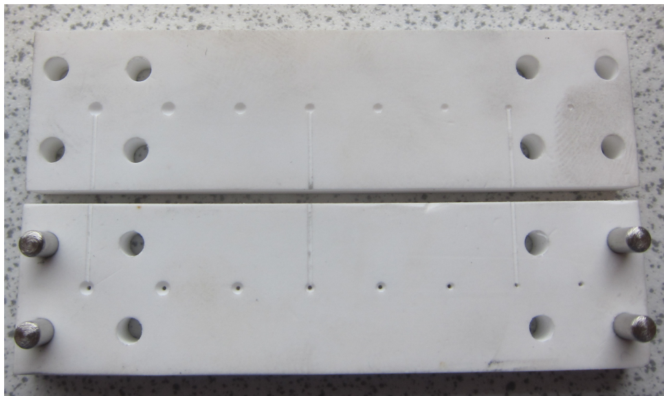
Figure 5.3: The image shows the cavities made of PTFE.
