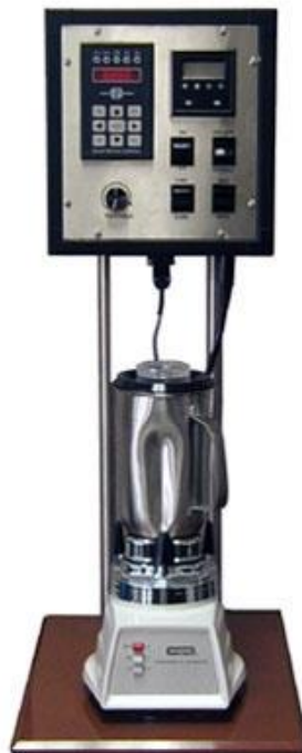
Figure 4.8. OFITE Constant Speed Blender used for preparing cement paste (OFITE, 2014).
