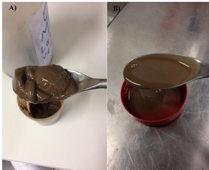
Figure B.1: A) OBM at 100°C (dehydrated), B) OBM at 50°C.
