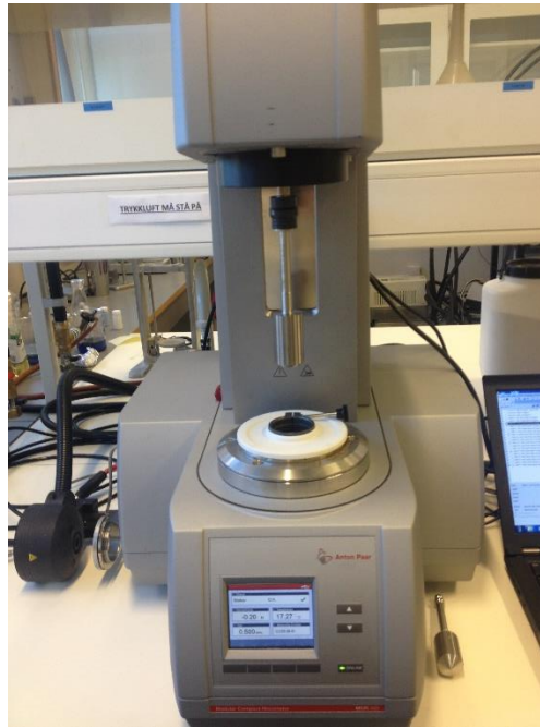
Figure 3.13: General view of the MCR with the viscometer measuring cell.
