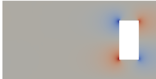
Figure 2.22: Examples of singularities in analysis using CCSC
