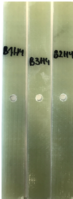
Figure 3.3: Coupons with circular holes (here, R = 4.0 mm).
