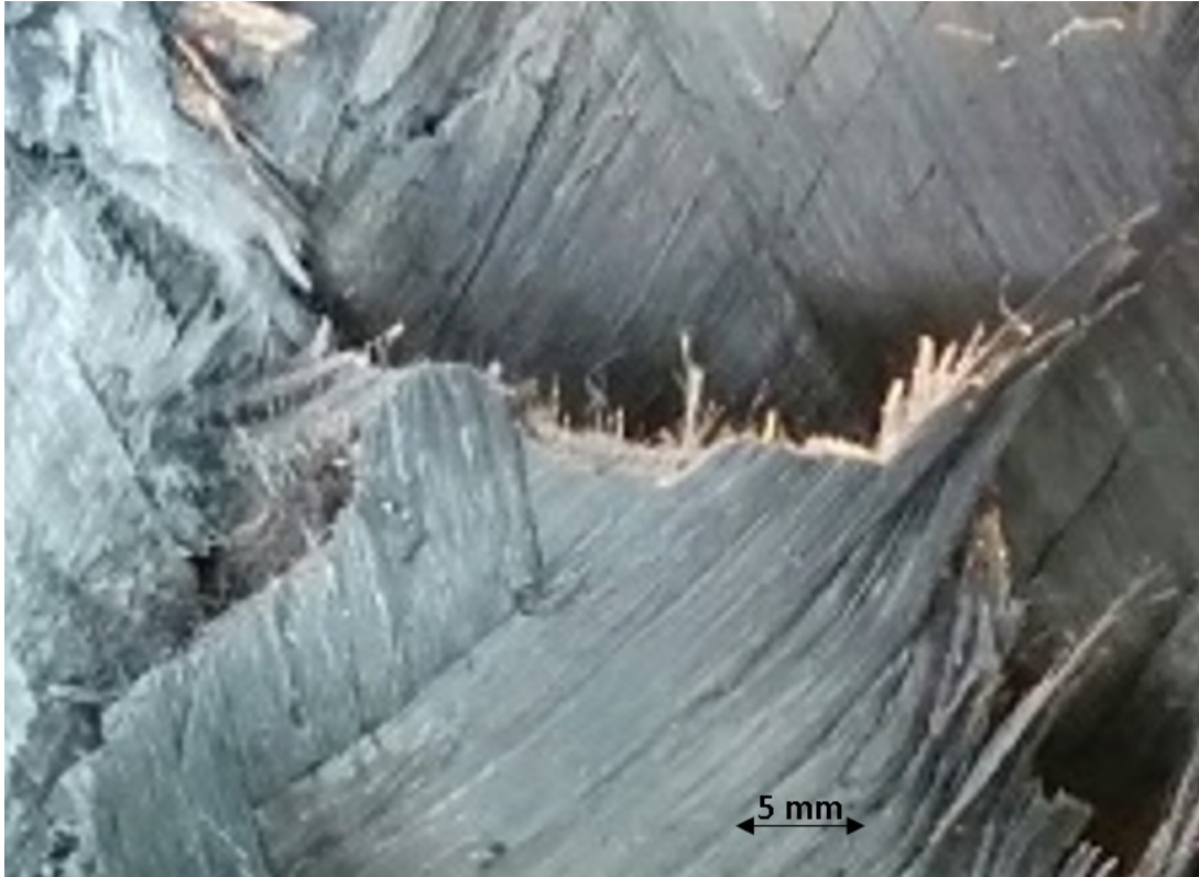
Figure 5.12: Shear failure of the SFRP6 hoop sample.
