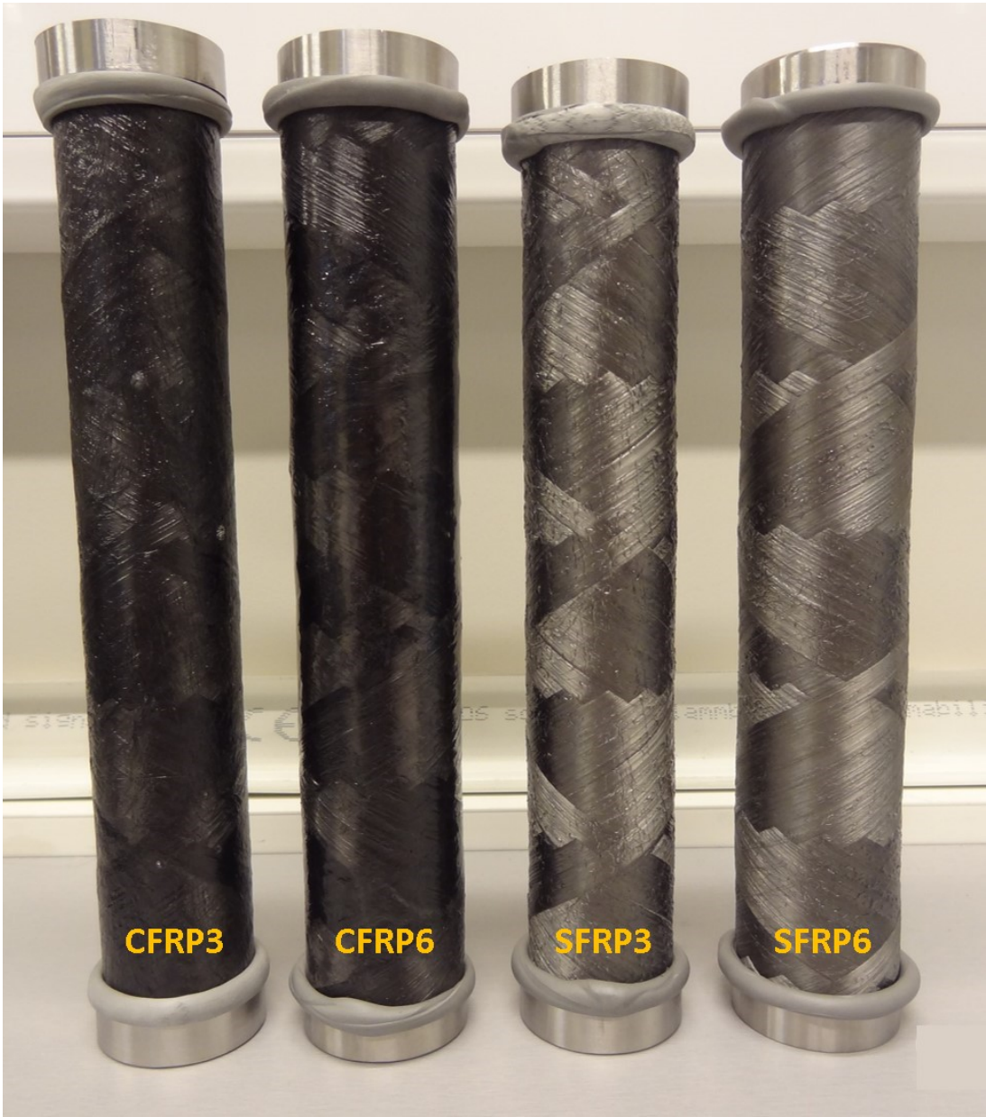
Figure 4.4: Assembled samples ready for buckling test with the end caps fitted into it with vacuum bag sealant tape.
