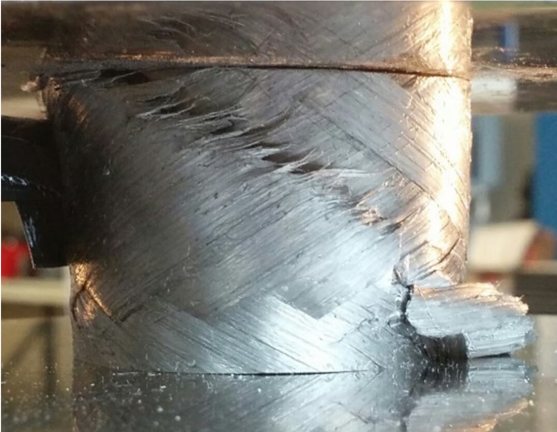
Figure 5.5: Failure and kink band formation during axial compressive loading of the SFRP3 sample.
