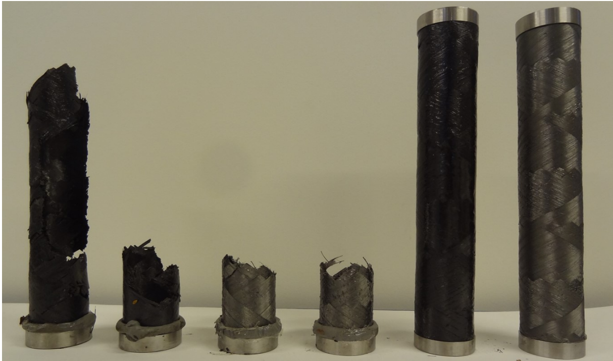
Figure 5.13: A picture showing the samples after external pressure test.
