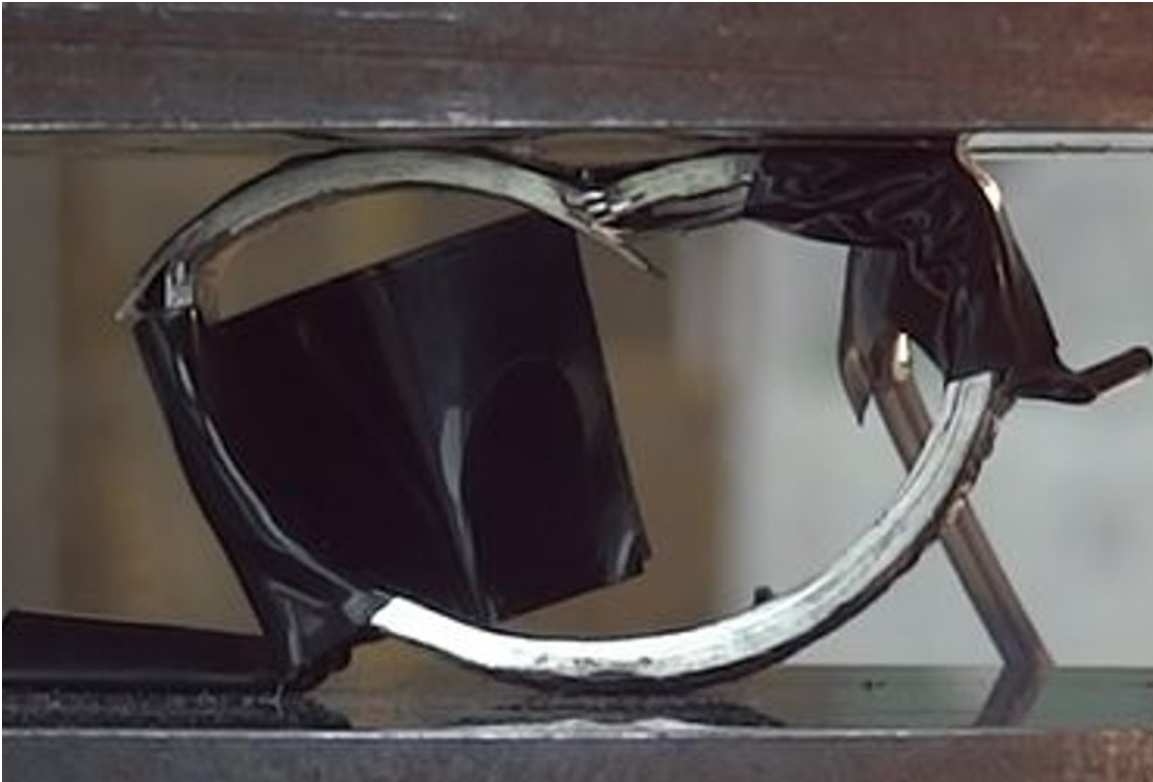
Figure 5.6: Failure of SFRP3 hoop sample.
