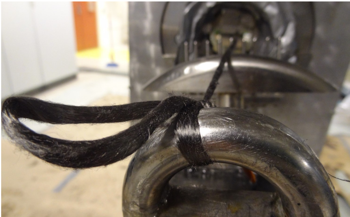
Figure 2.8: Steel fiber tied to the delivery by a simple double knot.
