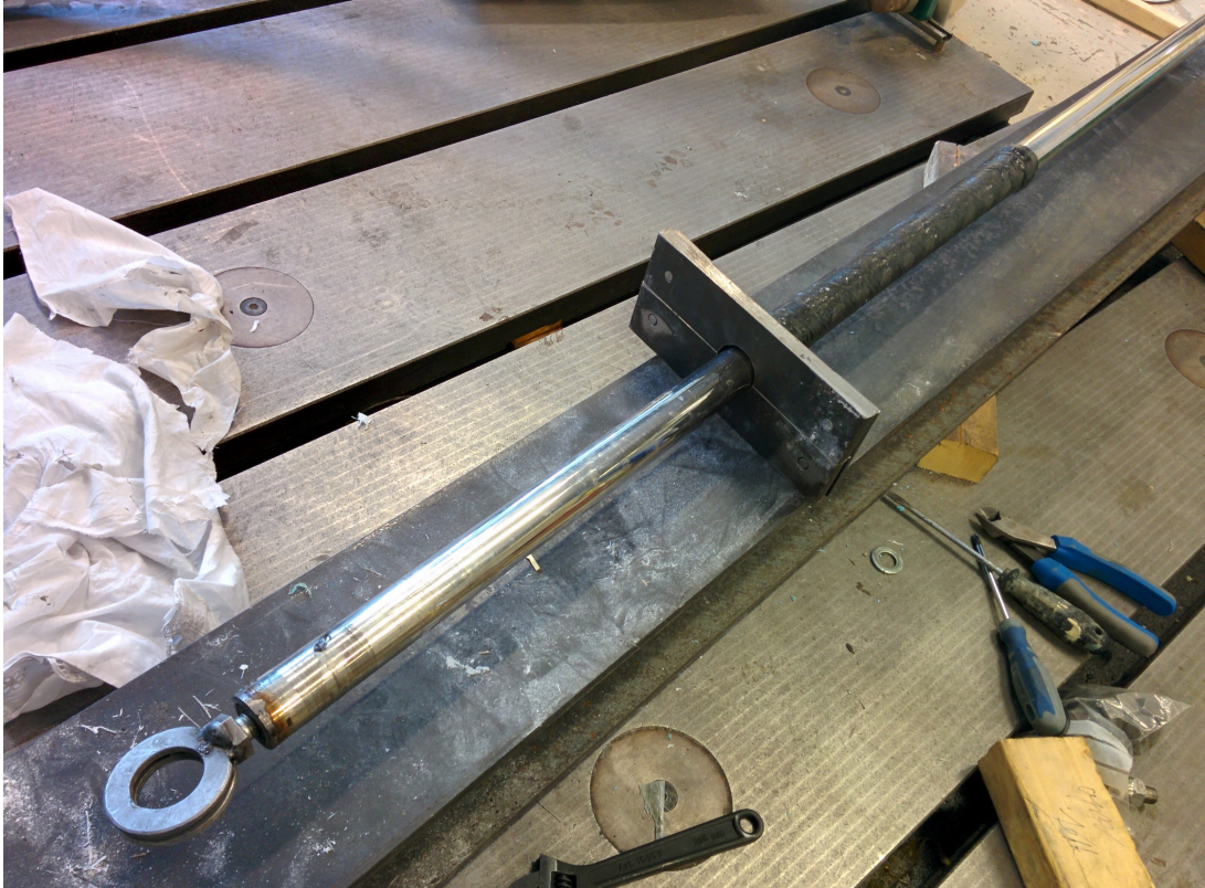
Figure 2.21: A picture showing the connection point for the lever chain hoist to the mandrel.
