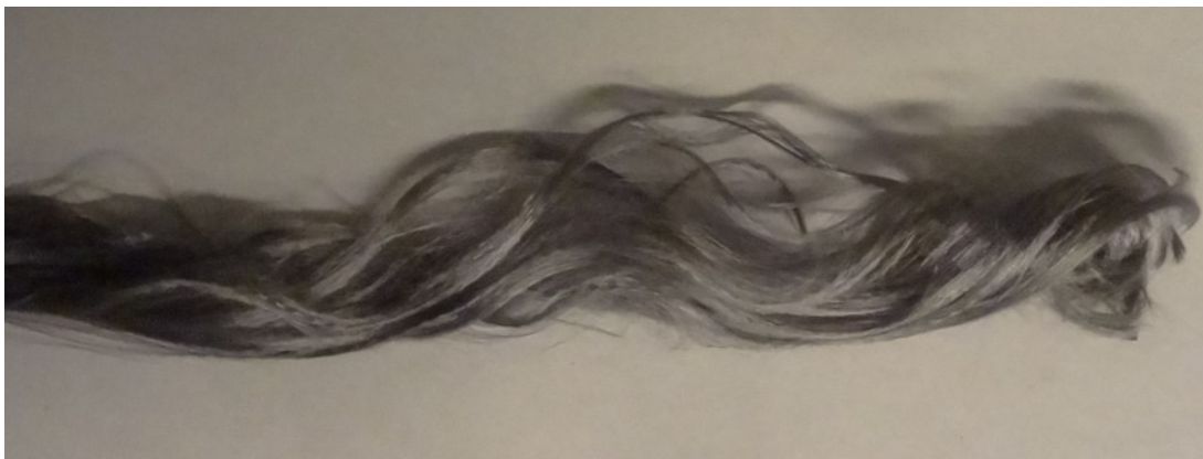
Figure 2.16: The picture shows that the broken fiber splits and tangles very easily.
