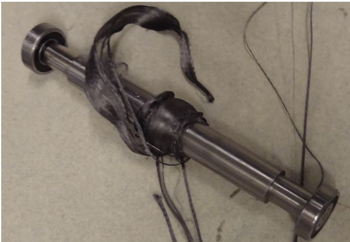
Figure 2.14: The broken fiber splits up and tangles around Roller A in the resin carriage.
