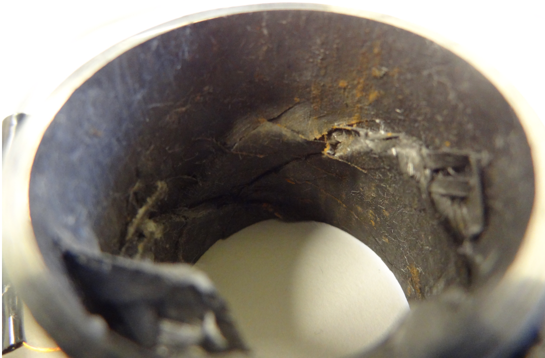
Figure 5.3: Failure of SFRP3 hoop sample.
