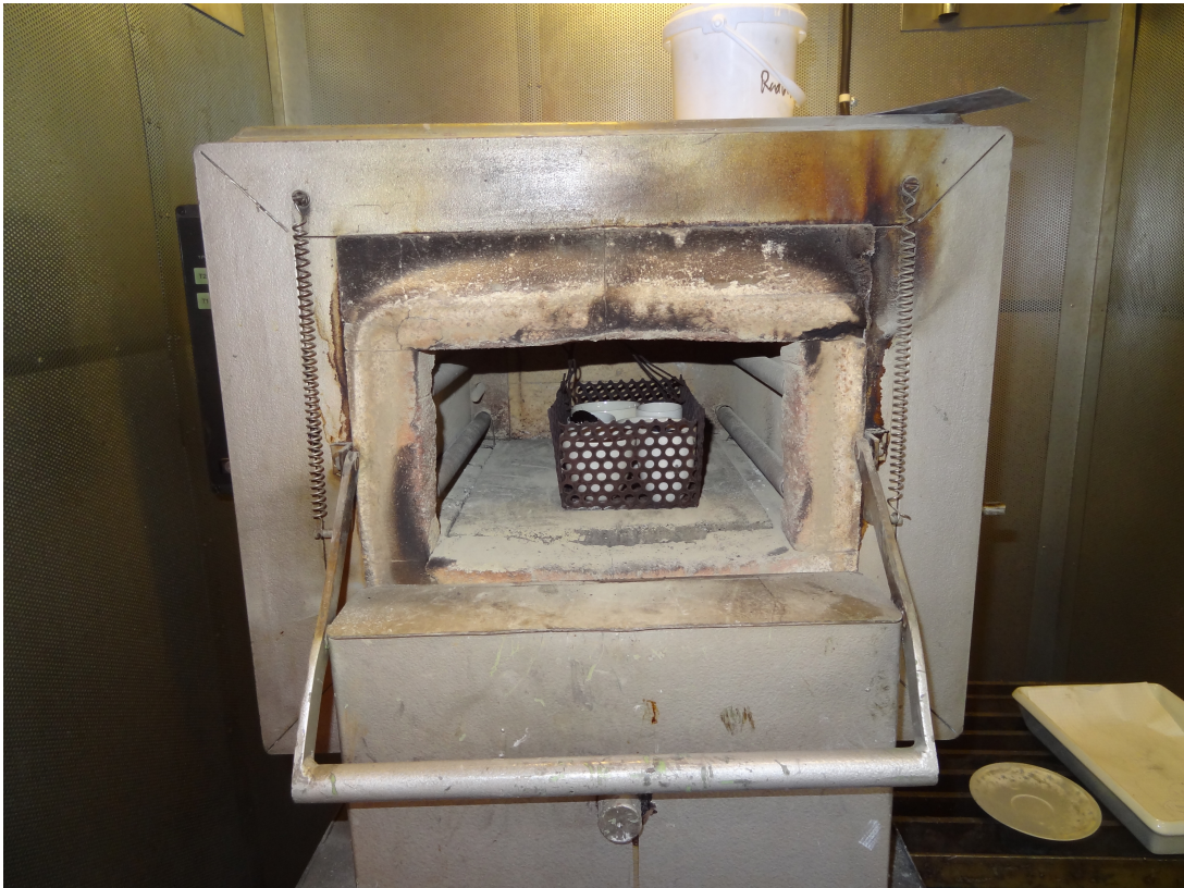
Figure 4.5: Samples in muffle oven ready for burn-off test.
