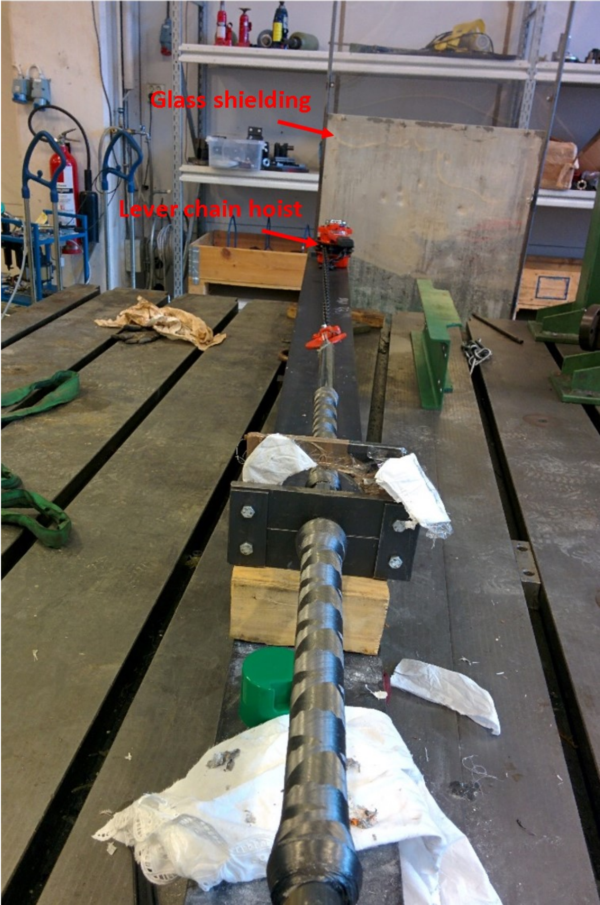
Figure 2.22: The picture shows the arrangement used to extract the pipes.
