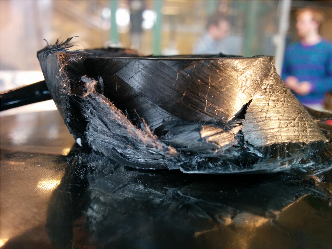
Figure 5.9: Failure of the SFRP6 axial sample.
