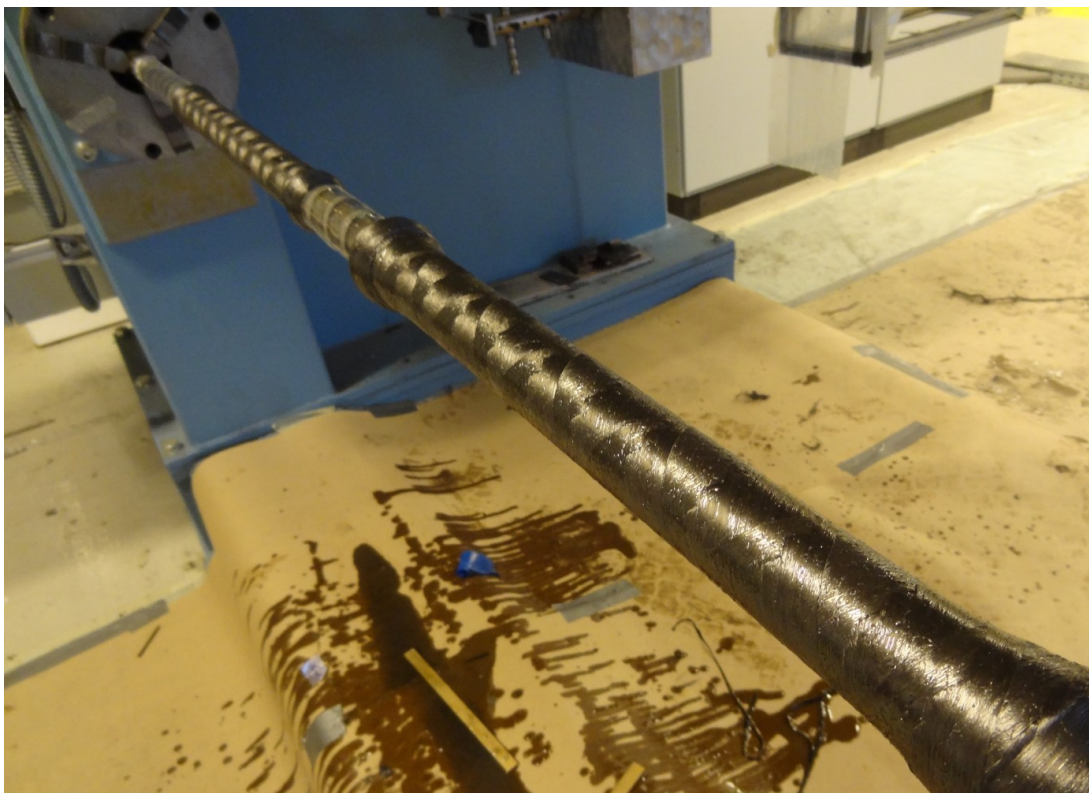
Figure 2.19: Mandrel rotating in winding machine for 24 hours to prevent resin migration after winding procedure is finished.
