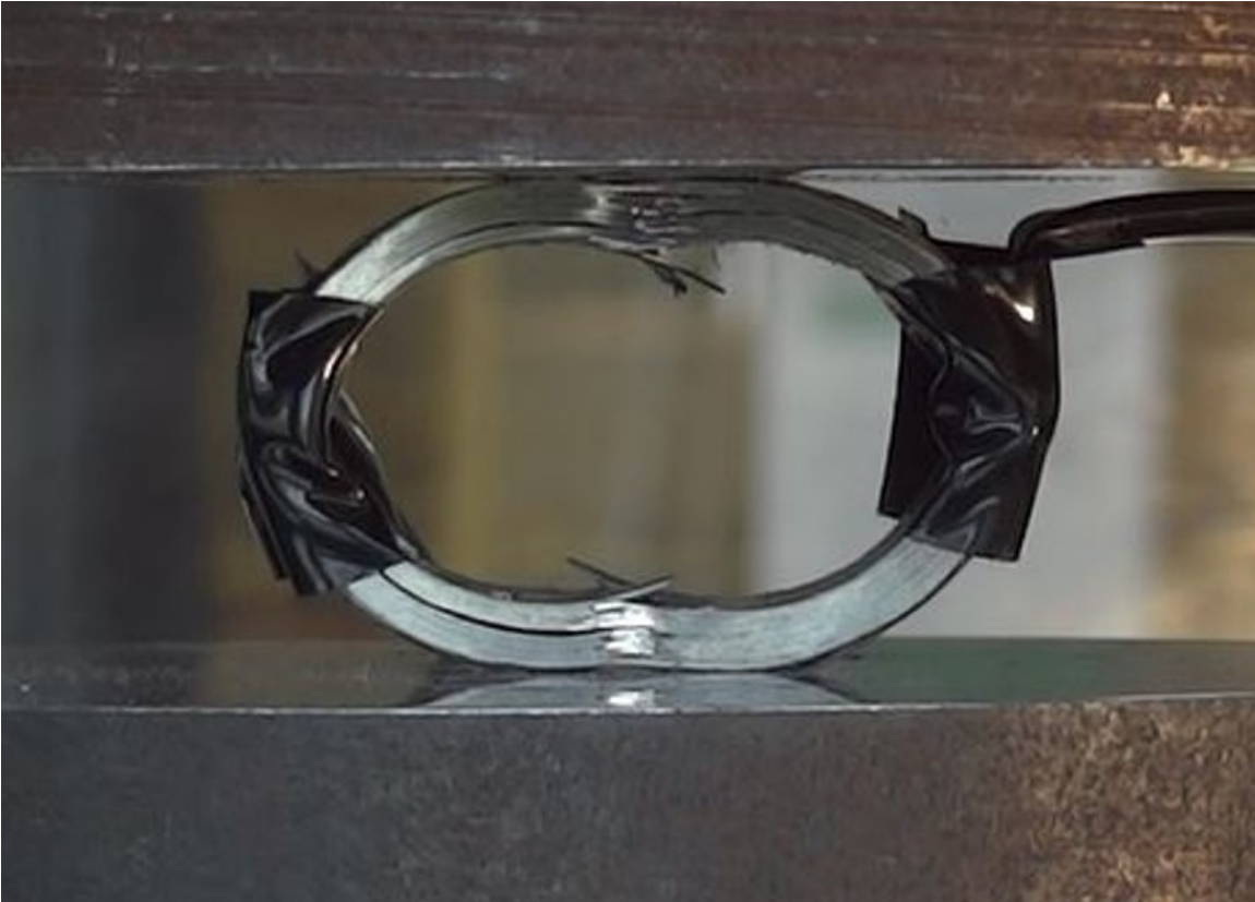
Figure 5.10: Failure of the SFRP6 hoop sample.
