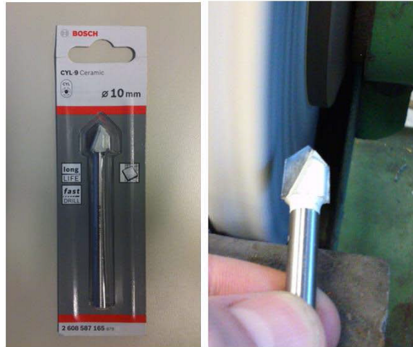
Figure 3: a) Bosch CYL-9 10 mm b) grinding of drill bit
