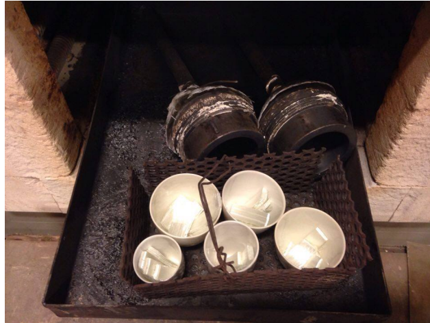
Figure 4.4: First burn-off test, accompanied with end fittings used in the filament winding process.
