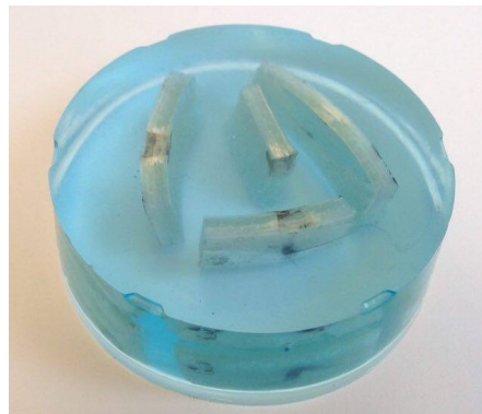
(b) Sanded epoxy block filled with samples.
