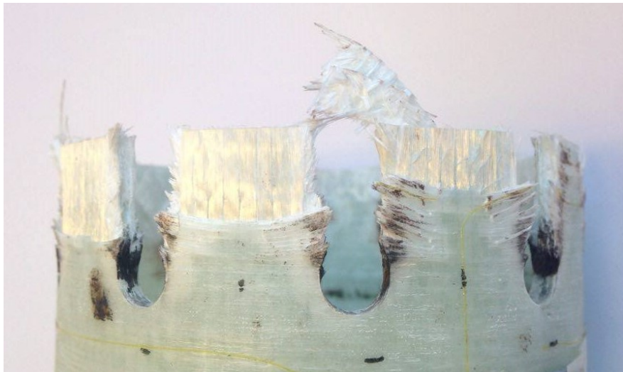
Figure 5.19: Sample ultimately failed due to shear out.
