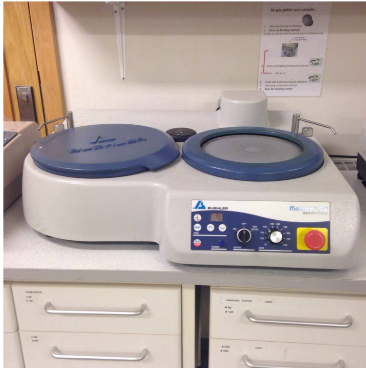
Figure 5: Sanding machines at Metallurgy lab at IPM.
