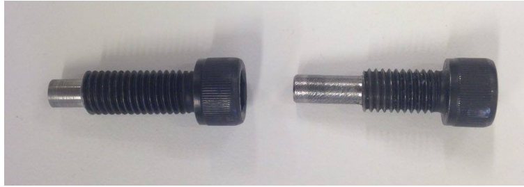
Figure 4.3: Old modified bolt (left) and new modified bolt (right). The difference is the distance the bolts have been machined in the z-direction. The diameter of the machined area is 7.9 mm on both bolts.
