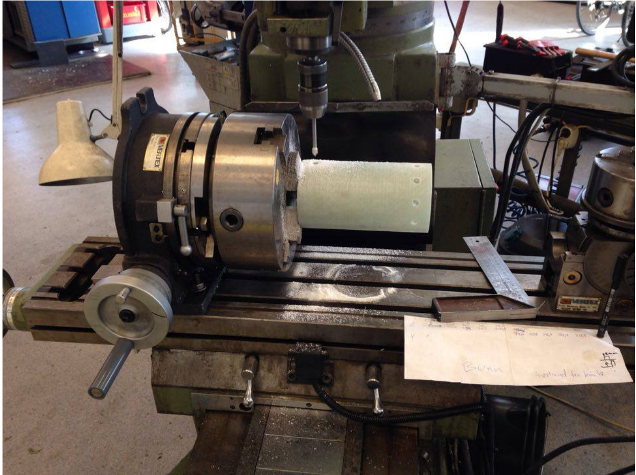
Figure 2: Photo of setup at milling machine. Including mill, chucks and tube mounted on the delehode.
