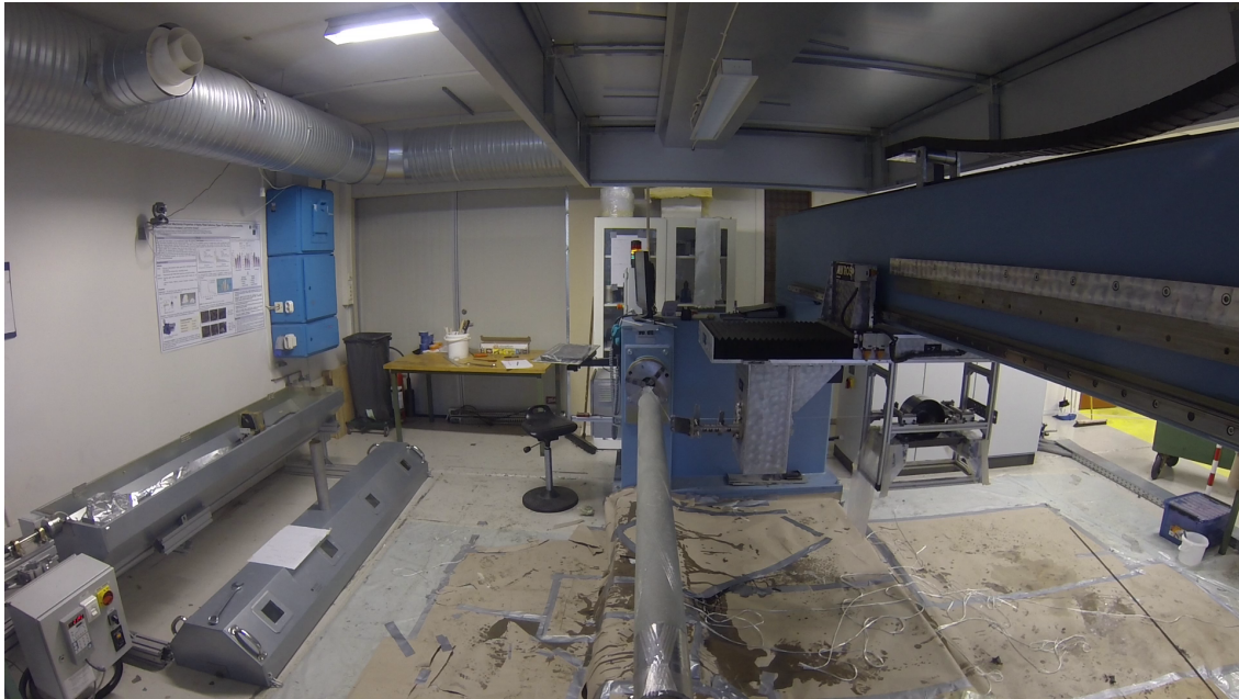
Figure 4.1: Filament winding of a two meter long tube on steel mandrel. The structure to the far left is the curing oven.
