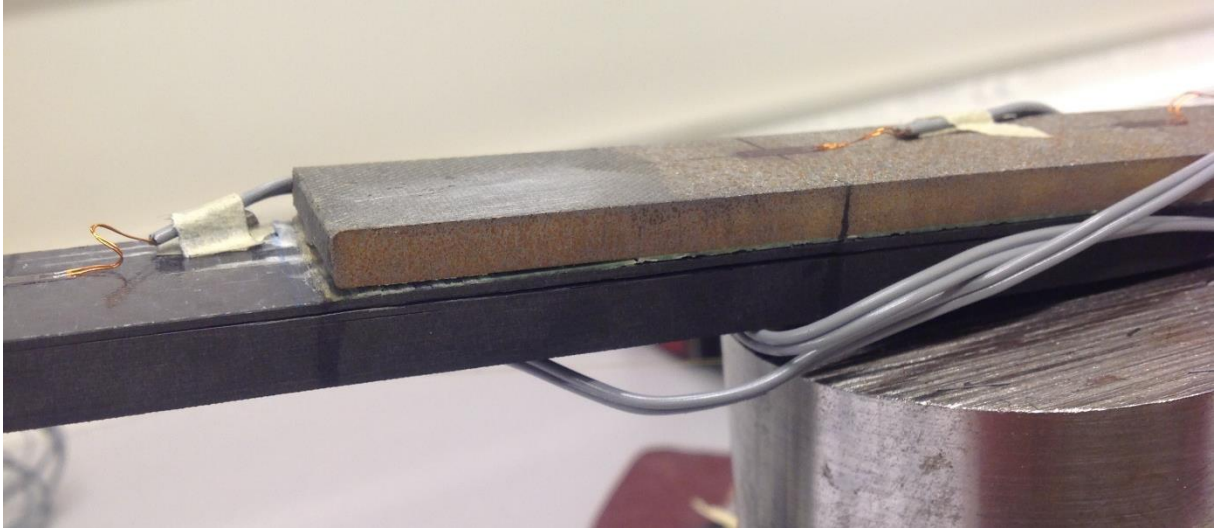
Figure 30: Debonding of steel adherend in HMC100_3
