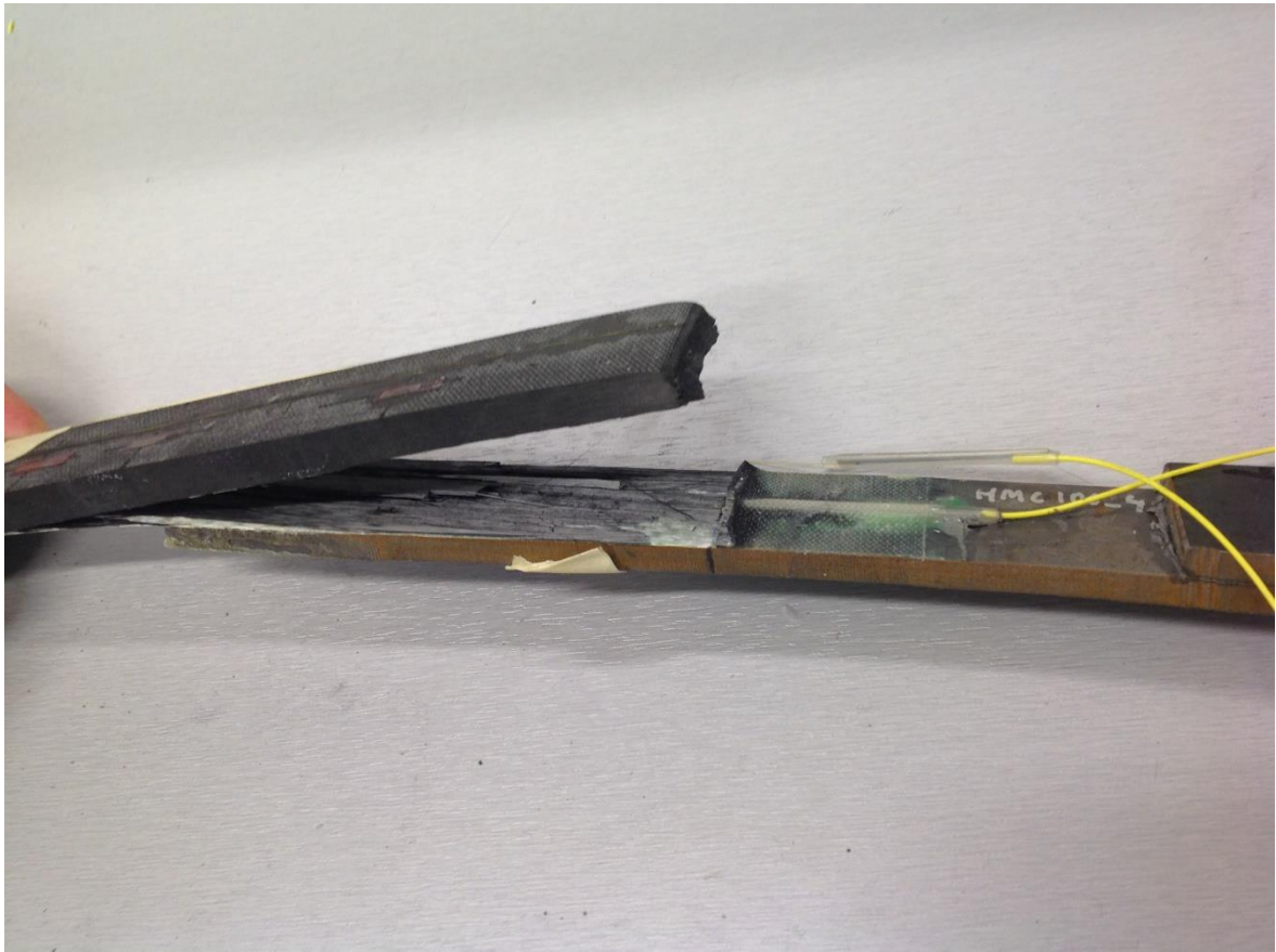
Figure 26: Failed sample HMC100_4 showing delamination
