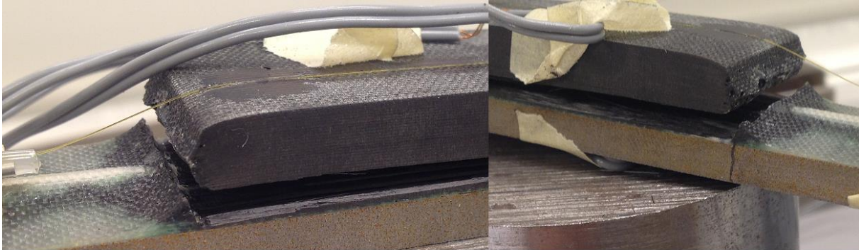
Figure 28: HMC100_2 with delamination in the left, and debonding progressing to delamination on the right
