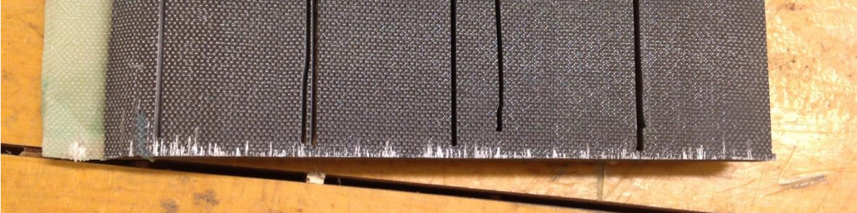
Figure 10: Water jet not fully cut through the laminate.
