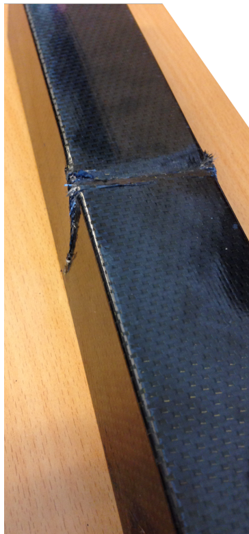
(b) Most fractured area, under loading point
