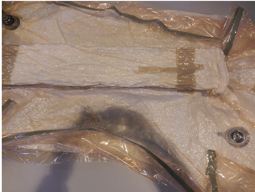
Figure 4.12: Bagging of I-beam
