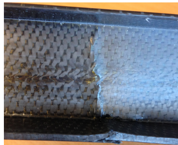
(c) Fracture under loading point
