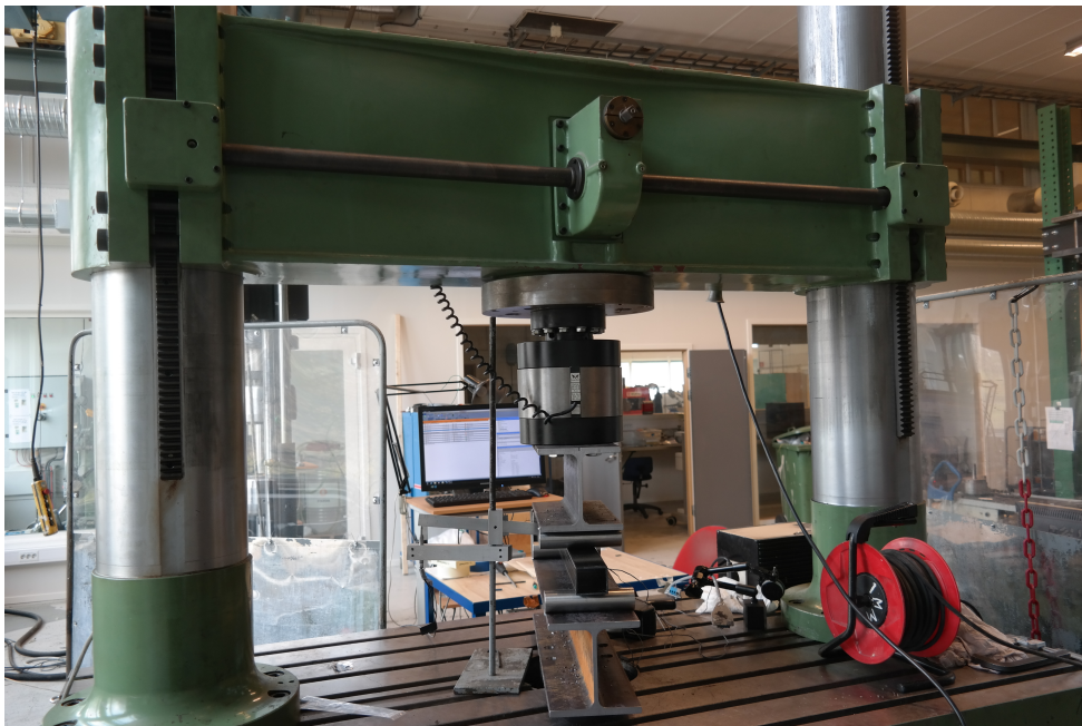
Figure 4.16: Test setup for four point bending test at IPM NTNU
