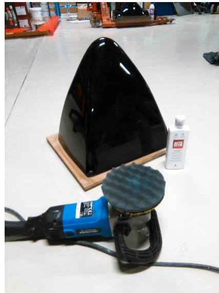
Figure 55 PU-foam mold ready for sealing and releasing
