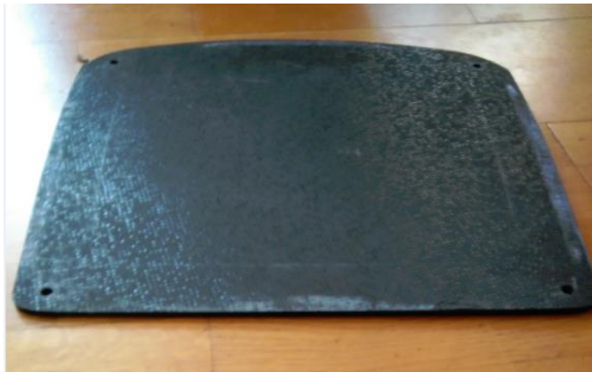
Figure 40 Finished carbon fiber anti-intrusion plate
