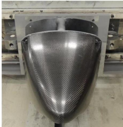
Picture 6 Impact attenuator frontal view
