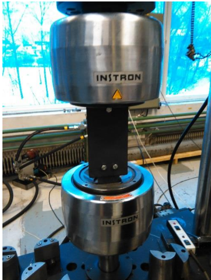
Figure 50 Attachment point test carbon fiber
