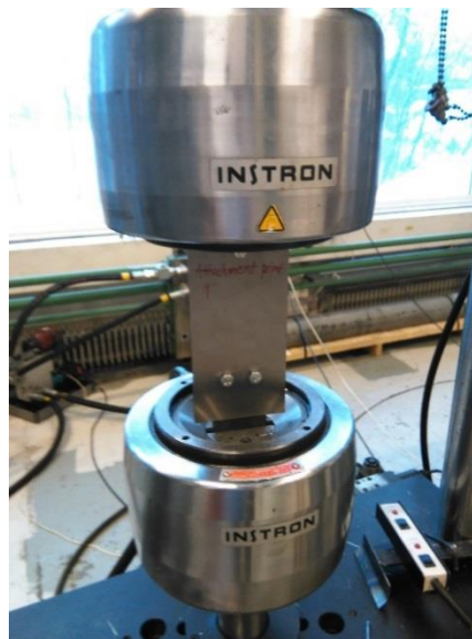
Figure 49 Attachment point test steel
