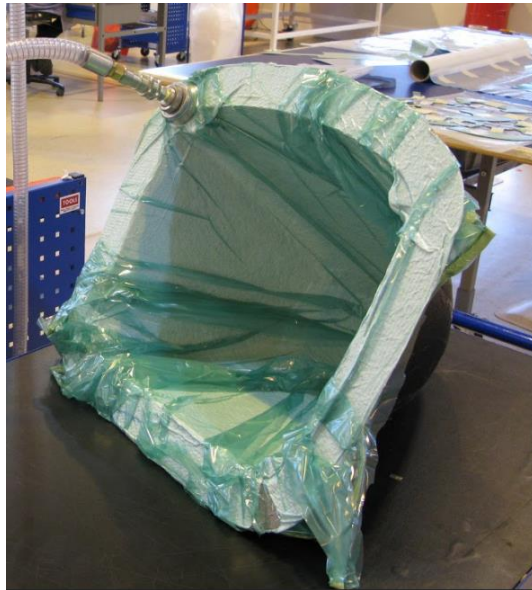
Figure 62 First crash nose in production
