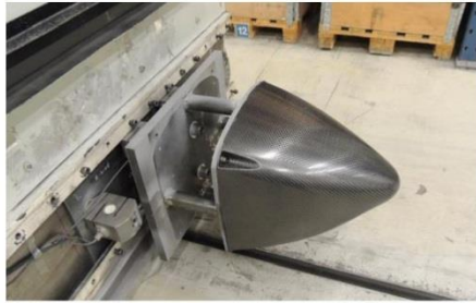
Picture 4 Impact attenuator on crash rig
