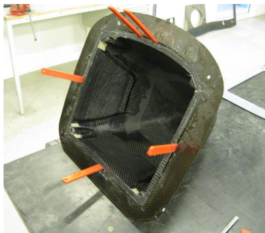
Figure 75 Finished crash nose during demould
