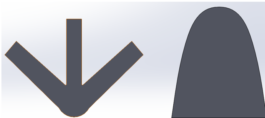
Figure 73 Plies used around bolt holes
