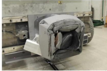
Picture 5 Impact attenuator post crash
