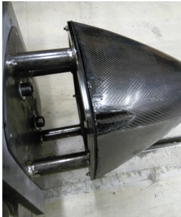
Figure 67 Epoxy used to cover dry areas
