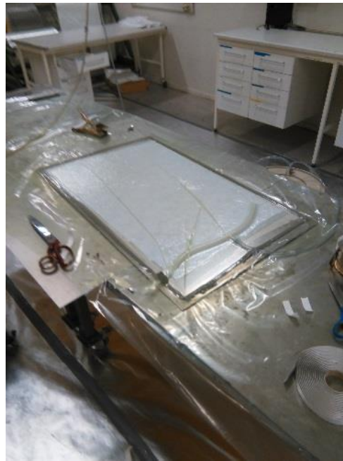
Figure 41 Debulking process. Laminate is put under vacuum to pack layers together
