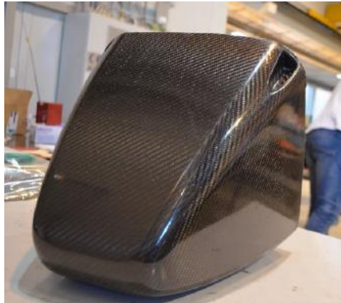
Figure 11 Crash nose from the 2015 car
