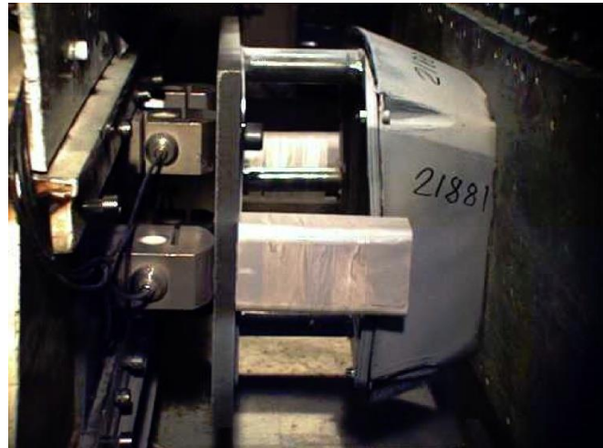
Figure 74 Top edge of crash nose going over the crash rig
