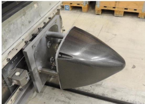
Picture 14 Impact attenuator as mounted on crash rig
