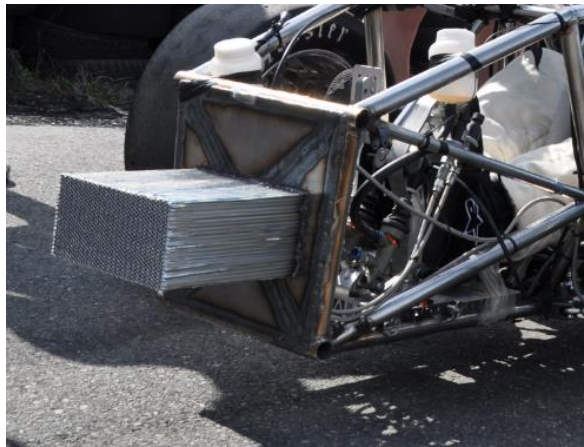
Figure 10 Revolve NTNU 2013 aluminum crash box mounted directly on the anti-intrusion plate
