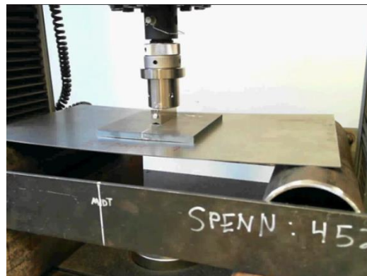
Figure 44 3-point bend steel
