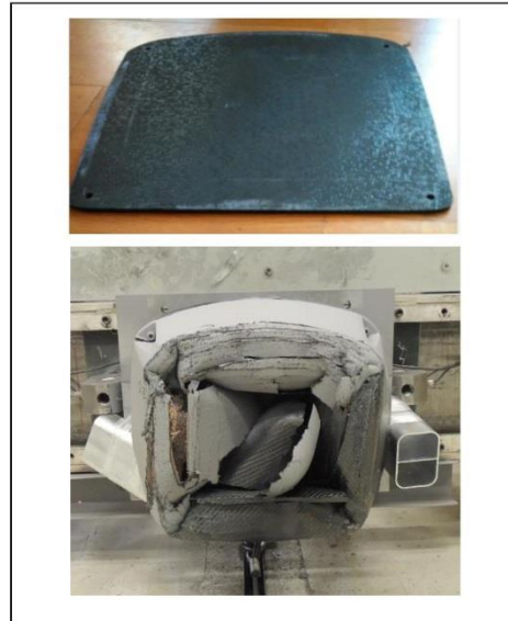
Figure 4: Attenuator after Impact
