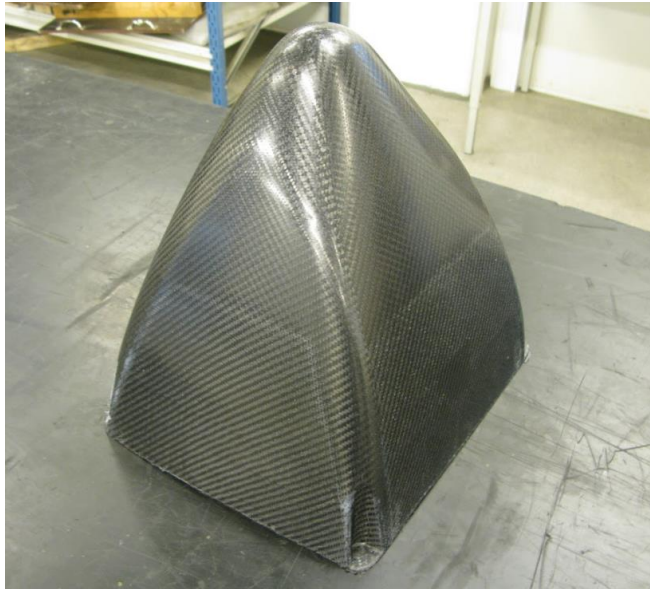
Figure 66 Dry areas around the core material due to poor core chamfering
