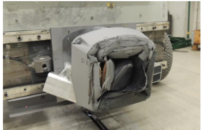
Figure 76 Second crash nose post-crash
