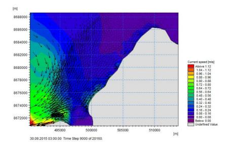
Figure 6.4: Current speed and direction at Bjørndalen caused by wind data from ECMWF and tidal variation
