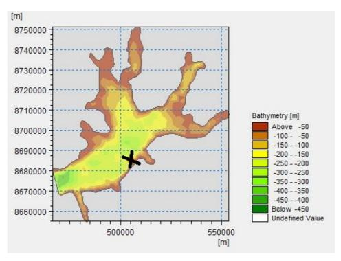
Figure 6.1: Mesh over Bjørndalen with the location the data is extracted from
