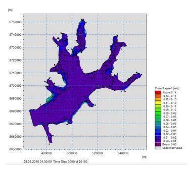
Figure 6.10: Current speed in Isfjorden with wind input from ECMWF and tides are neglected
