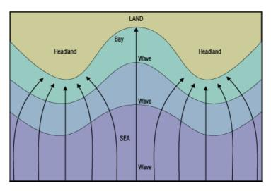
Figure 2.6: Illustration of waves refraction(Carleton, 2016)
