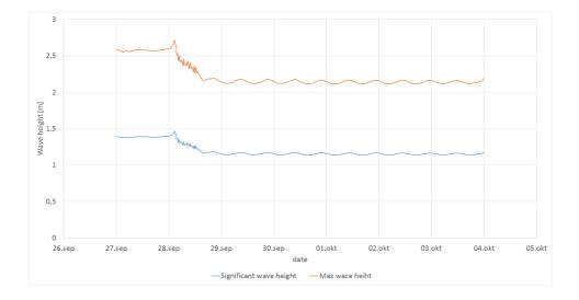
Figure 6.22: Wave height at Bjørndalen when wind is neglected
