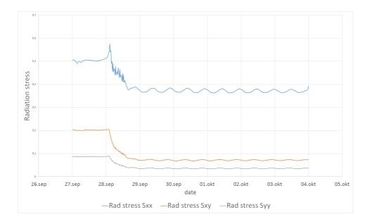
Figure 6.24: Radiation stresses at Bjørndalen when wind is neglected
