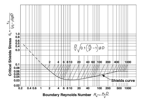
Figure 2.7: Shields Diagram(MIT, 2015)
