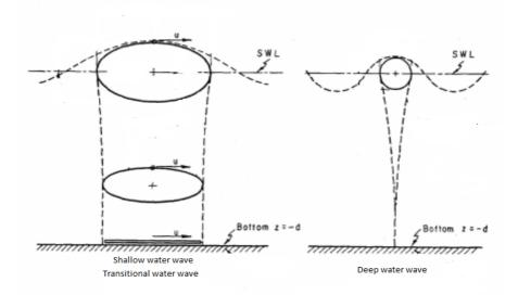
**Figure 2.4:** Water particle motion in shallow water and deep water. Based on figure(Krogstad and Arntsen (2003))
