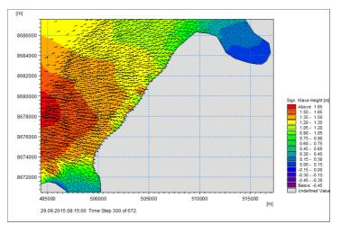
Figure 6.14: Significant wave height at Bjørndalen
