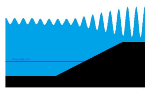
Figure 2.5: Illustration of waves shoaling
