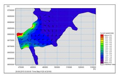
Figure 6.6: Current velocity and current direction at Isfjorden using data from ECMWF
