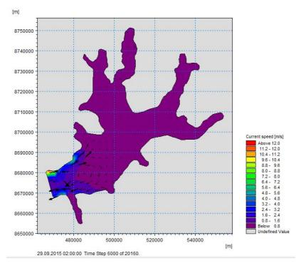
Figure 6.3: Current at Bjørndalen with wind data from NMI
