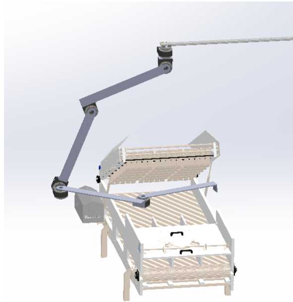
Figure 3.13: A long reach is possible with a modular robot.
