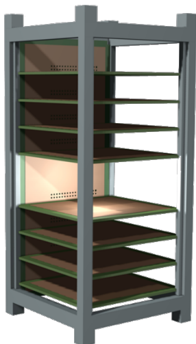
Figure 1.1: The figure shows a 3D model of the proposed backplane design used in NUTS.
