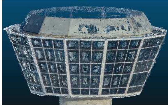
Figure 15 - Prism and roof, depicted using all edited photos in default processing. White pixels are not removed noises.
