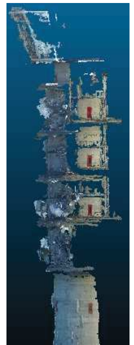
Figure 18 - Overall view for dataset made of half of the taken, original photos in slow processing mode.
