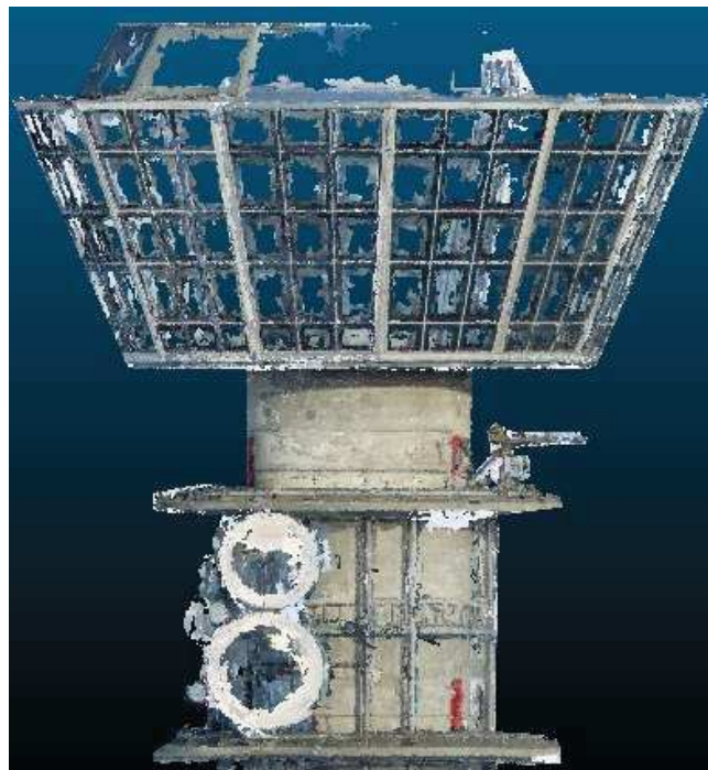
Figure 20 - Highly dense point cloud. The roof is badly depicted.
