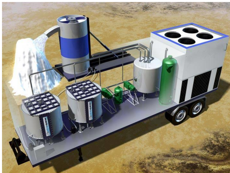
Figure 3-4 SnowGen, showing the ice slurry generator in the container and the snow separator behind (Tucker, 2014)
