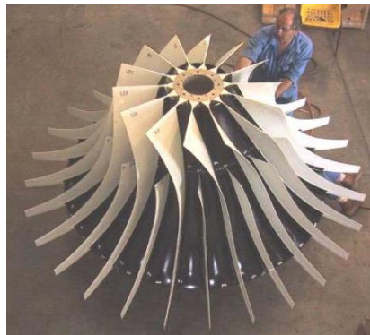
Figure 4-2 Radial compressor used in a vacuum ice maker (Ophir, 2007)
