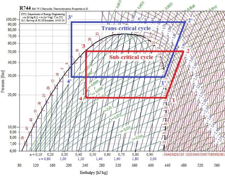
Figure 4-3 Simple trans-critical and sub-critical CO 2 cycle
