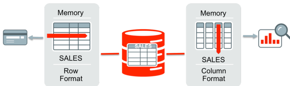
Figure 10.1: The Oracle Database dual format. Data is stored as both rows for transactional performance, and columns for analytical performance. (Adapted from [45])
