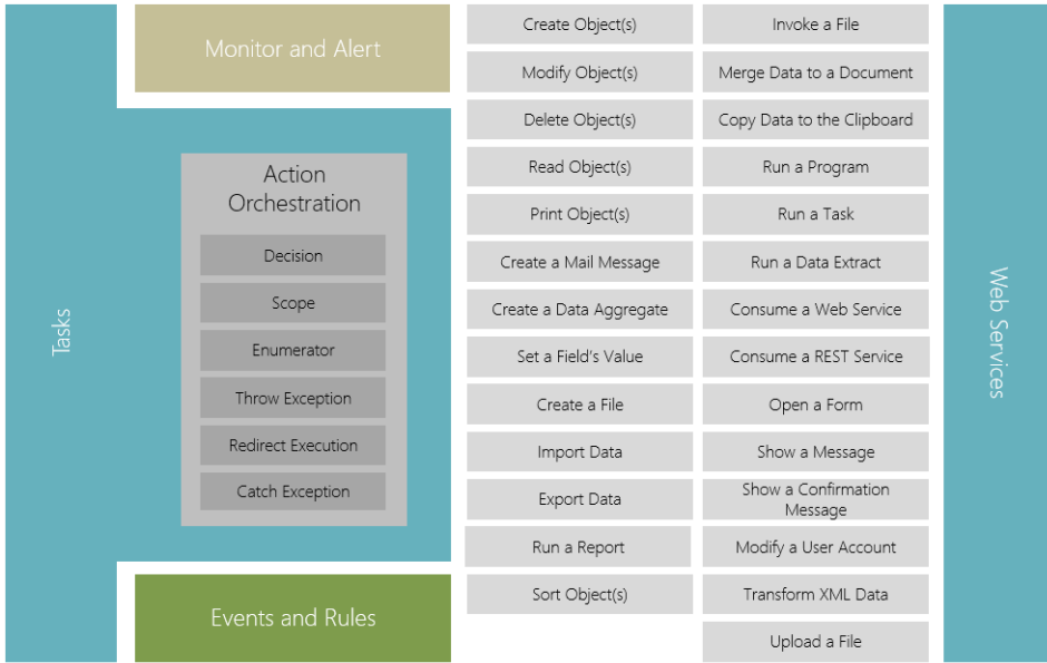
Figure 4.3: The logic layer in Genus App Platform . Here, tasks and effects are specified through action orchestration. Tasks contain programming-like constructs and is composed of a wide variety of actions. (Adapted from [32])
