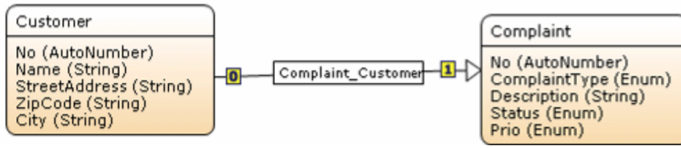
Figure 2.3: Class diagram in Mendix . (Adapted from [34])
