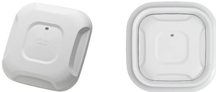
Figure 2.3: Left is a Cisco Aironet AP 3700 series. Right is the same AP with the Hyperlocation module installed. ( www.cisco.com )
