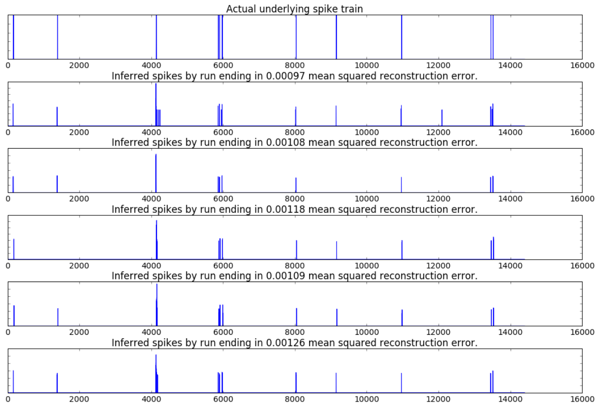
Figure 5.2: The top plot shows the actual target spikes underlying the observed signal. The five plots under show what the ANN thought the spike train looked like given the mean squared error it achieved. These five ANNs are the ones who got the lowest training error, corresponding to the left-most bar, in figure 5.1
