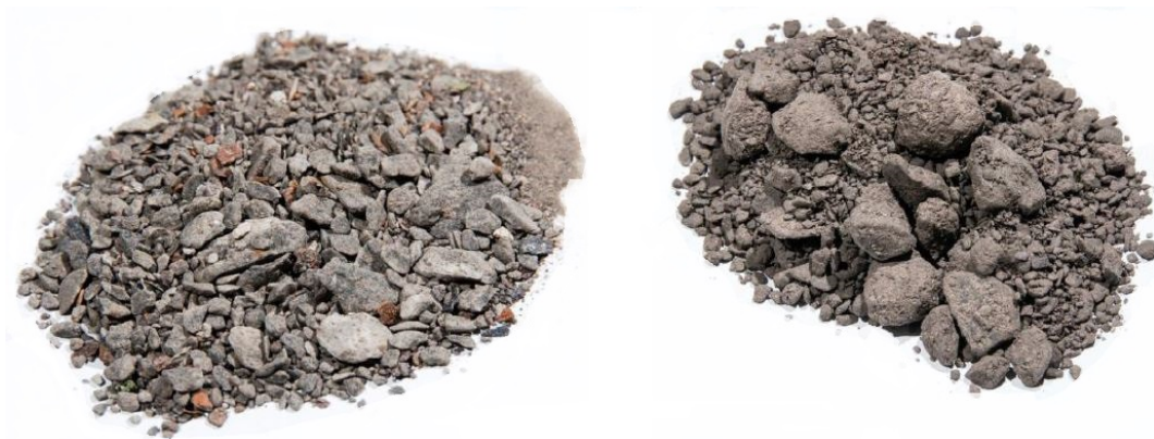
FIGURE 5.25: Large cuttings produced by CDE equipped PDC bit (right) greatly enhances geological/petrological evaluation [36].
