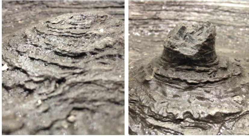
FIGURE 5.24: Full scale drilling validated FEA-model with conventional PDC bit (left) and new CDE equipped bit (right) [36].
