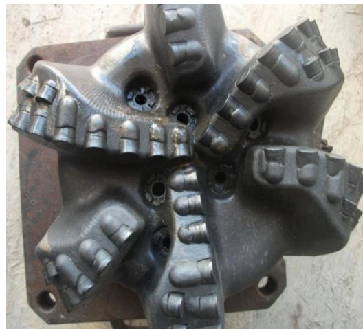
FIGURE 5.29: Standard PDC bit used in a offset well in Iraq [36].
