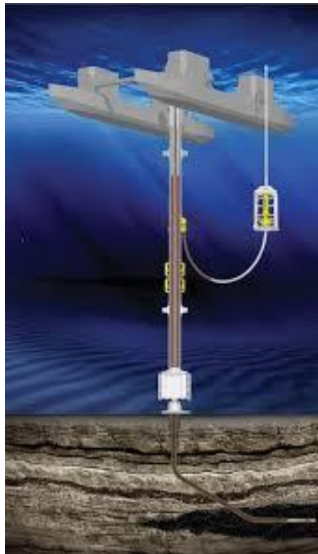
Figure 4.16: Low Riser Return System [50].
