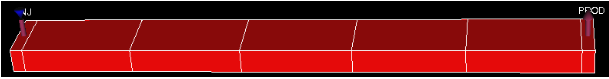
(b) Coarse Grid Model (Grid Block Size = 180m*100m*40m)
