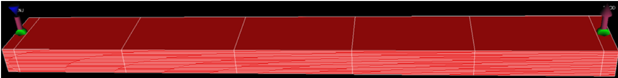
(b) Coarse Grid Model (Grid Block Size = 180m*100m*2m)
