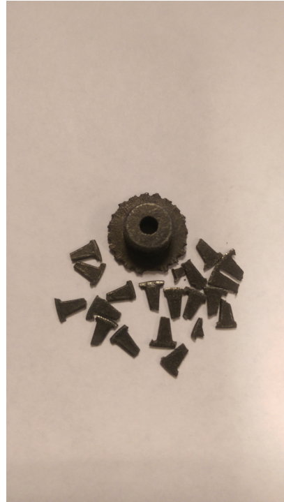
(a) The encoder disc as mounted on the (b) The encoder disc and all its fragments rotating shaft
