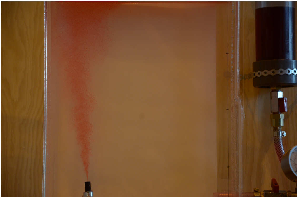
Figure A.16: Testing in tank 2 using paraffin and with a pressure drop of 0.3 bar across the nozzle
