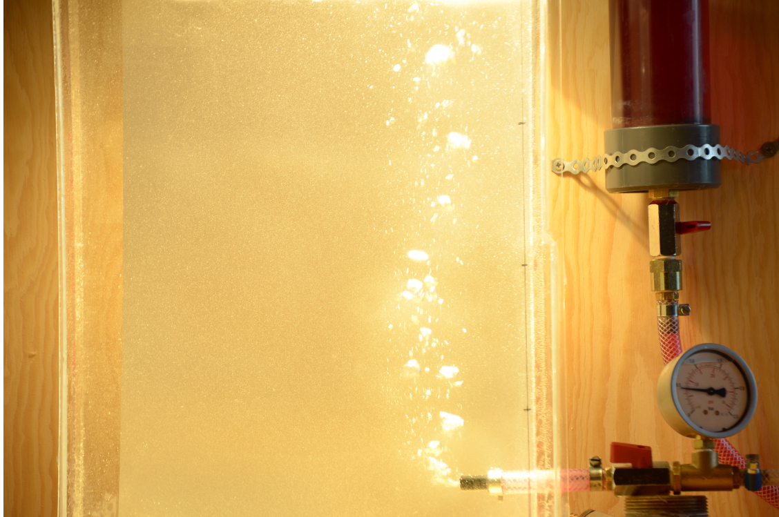
Figure A.17: Testing in tank 2 using air and with a pressure drop of 0.5 bar across the nozzle
