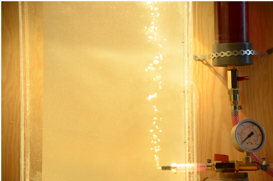
Figure A.18: Testing in tank 2 using air and with a pressure drop across the nozzle just enough to give air flow
