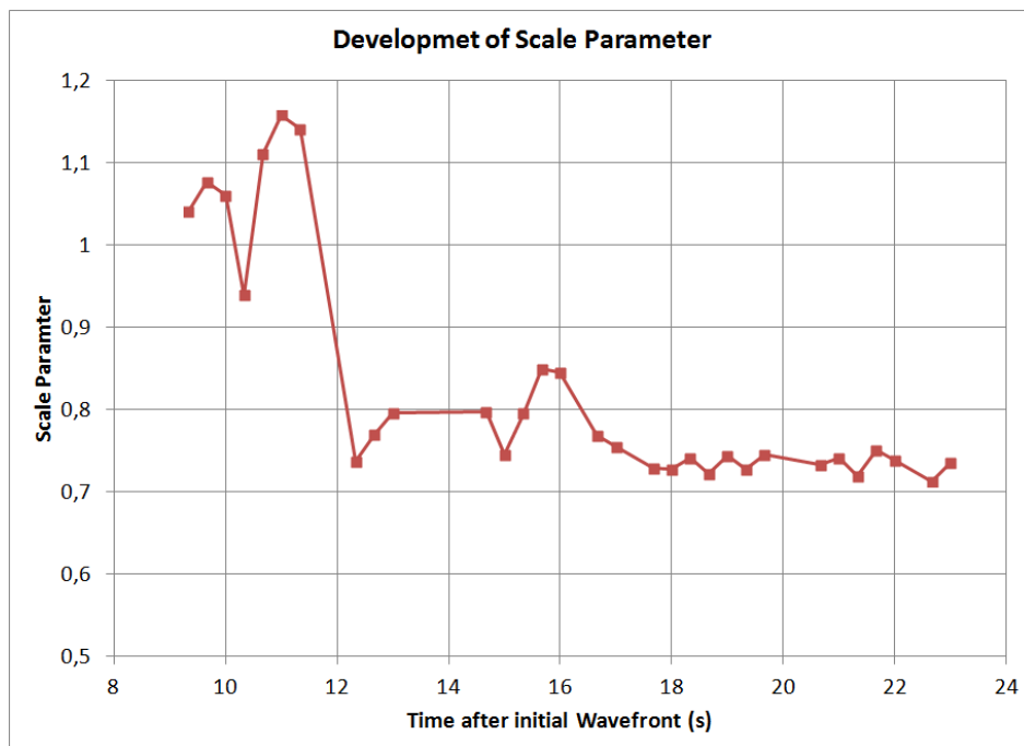
Figure 4.6: Log-normal scale parameter for droplets vs time after wave front for test condition seven
