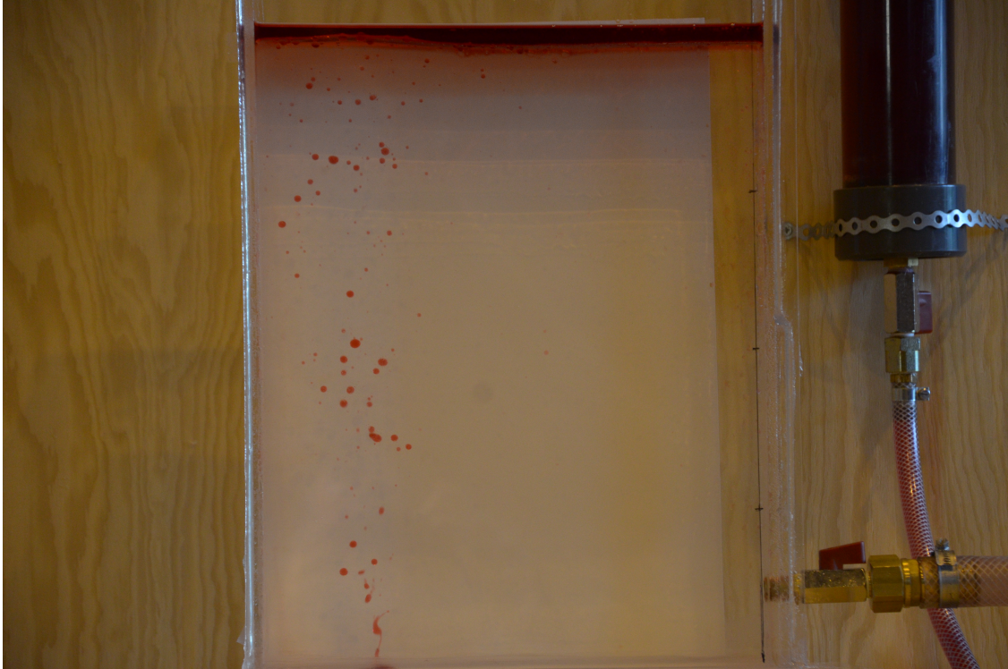
Figure A.7: Testing in tank 2 with a pressure drop of 0.5 bar across the valve and pump voltage 11.5 V
