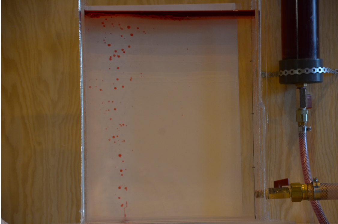
Figure A.5: Testing in tank 2 with a pressure drop of 0.5 bar across the valve and pump voltage 10.5 V
