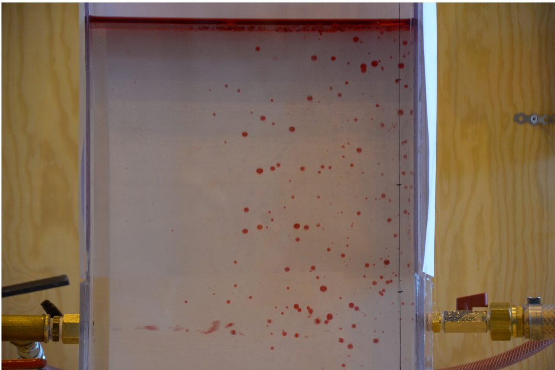
Figure A.2: Testing in tank 1 with a pressure drop of 1.0 bar across the valve and pump voltage 13.0 V
