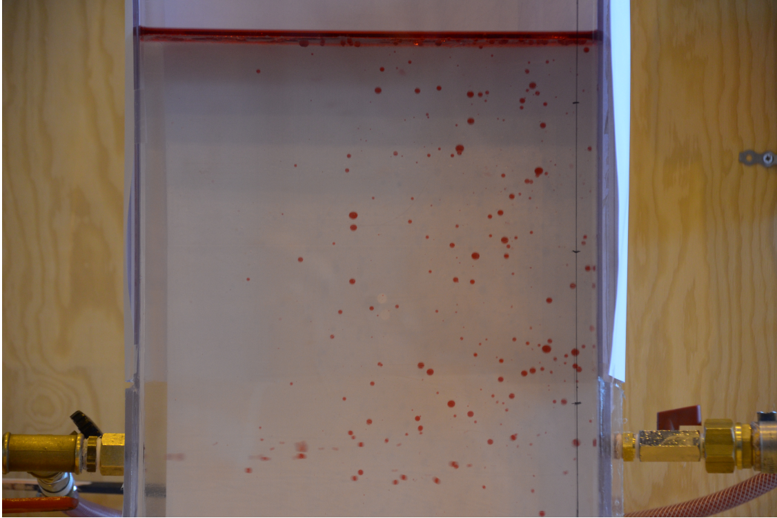
Figure A.1: Testing in tank 1 with a pressure drop of 0.5 bar across the valve and pump voltage 13.0 V
