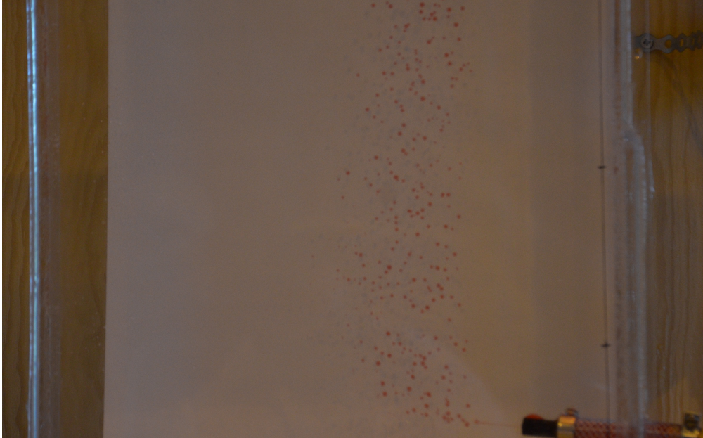
Figure 3.9: Image of oil injected horizontally through a nozzle with a pressure drop of 0.8 bar
