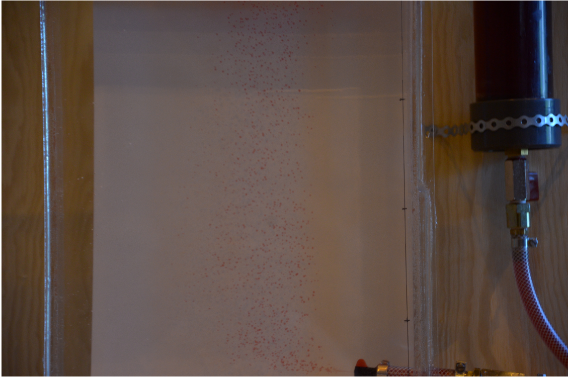
Figure A.13: Testing in tank 2 with a pressure drop of 1.0 bar across the nozzle
