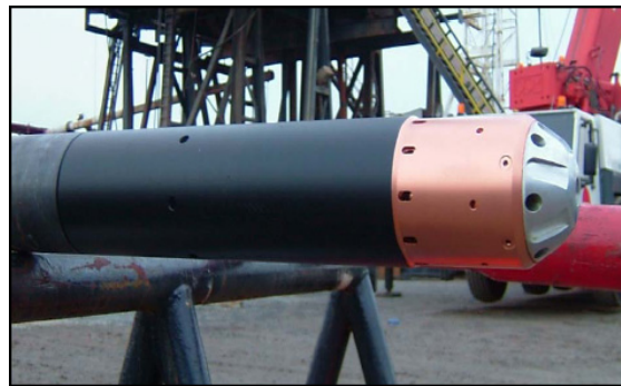
Figure 3.13 Flow Diversion Shoe (Howlett et al., 2006)
