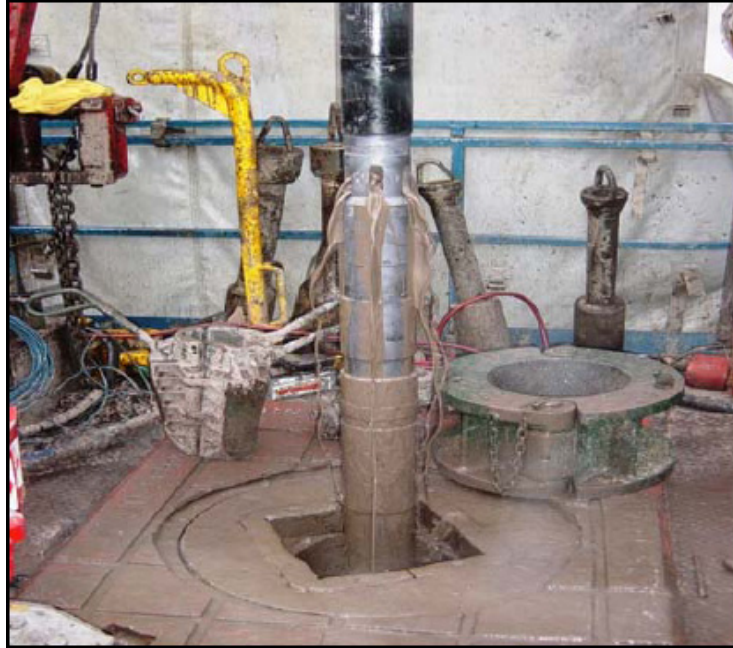
Figure 3.15 Mud flow from inner annulus (Howlett et al., 2006)
