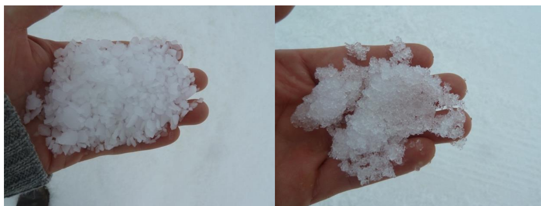
Figure 23: The picture on the left shows fresh snow out of the SF100. The picture on the right shows the snow after a few days in the tracks. Both pictures are taken at Idrefjäll, Sweden.
