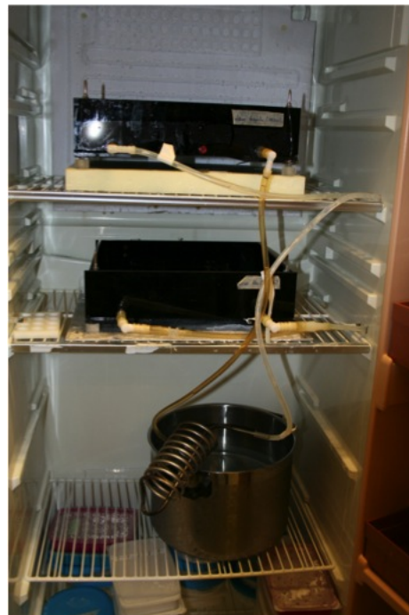
Figure 3.3: The setup during electrophoresis. The electrophoresis tank (on the top) was placed in a refrigerator and the electrophoresis solution passed through heat exchanger (60 cm below the electrophoresis tank) in ice/water during electrophoresis. Photo taken from the Department of Chemicals and Radiation at Norwegian Institute of Public Health, in Oslo, Norway.
