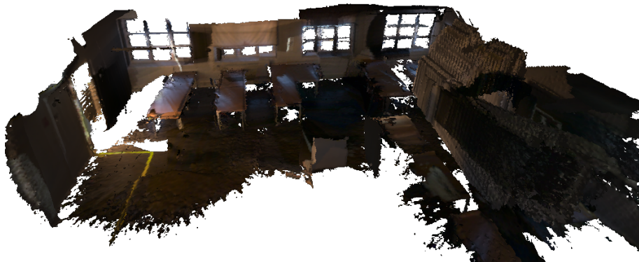
Figure 9: 3D representation of a room mapped using Project Tango Constructor
