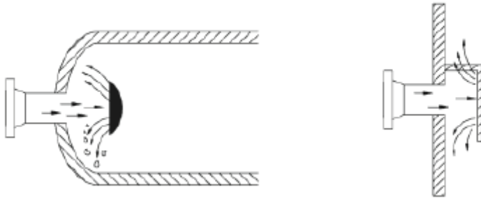
Figure 2-4: Showing examples of diverter plates (ken and Maurice 2008)
