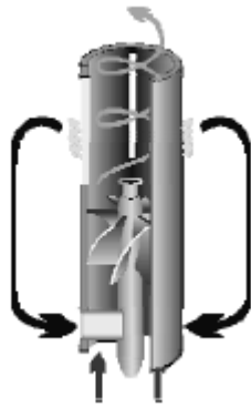
Figure 2-18: Showing spiral-flow demister (Yaojun 2009)
