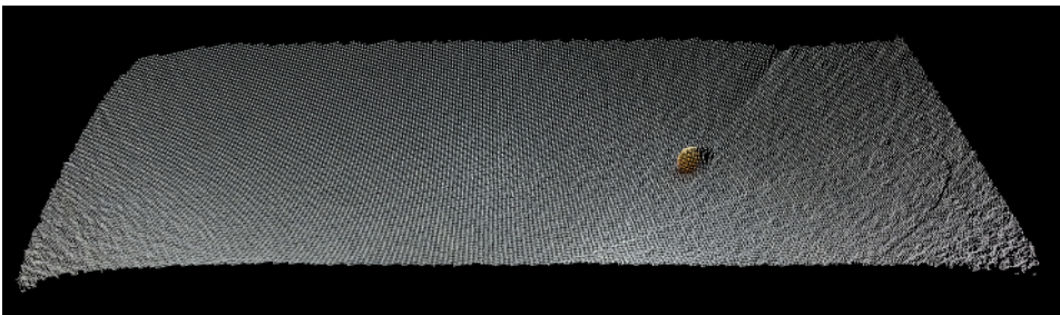
Figure 4.4: A point cloud of 49 396 points showing a ping-pong ball placed on the floor. For a random sampling strategy it would require approximately 7 000 000 times more iterations to detect the sphere, compared to the suggested sampling strategy. (Obtained with the Kinect for Xbox One)
