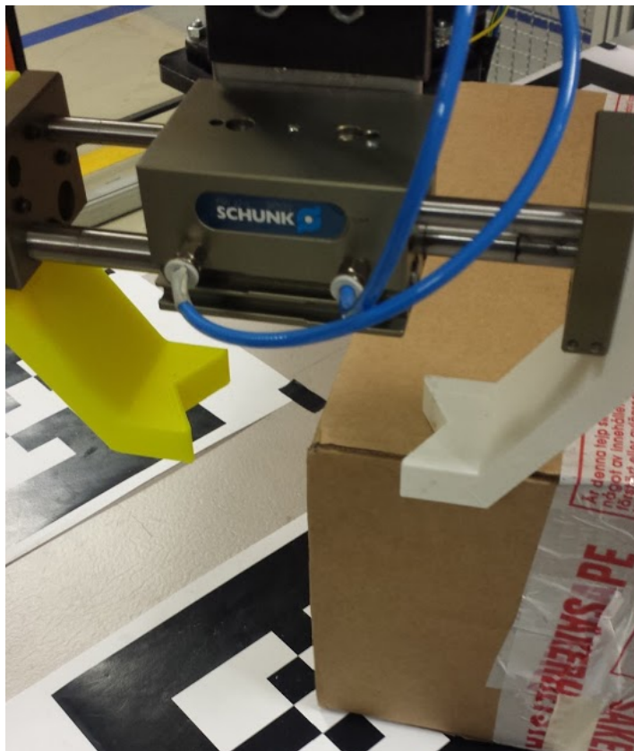
Figure 5.19: Robot manipulator placed directly above the found objects origin.
