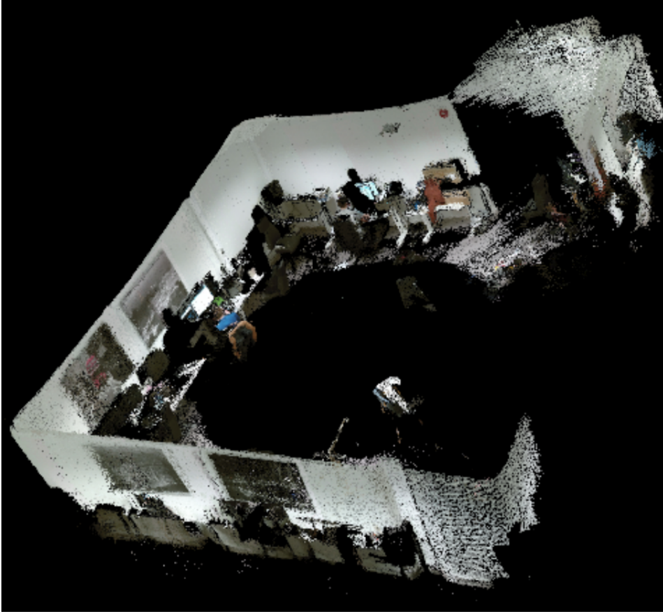
Figure 5.9: The reconstructed office room using a general registration approach with multiple point clouds.
