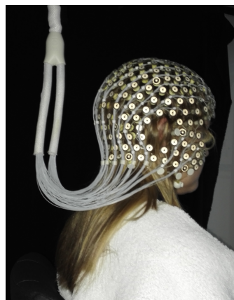
Figure 28.: The 256-electrode GSN net when mounted on the head of a participant.
