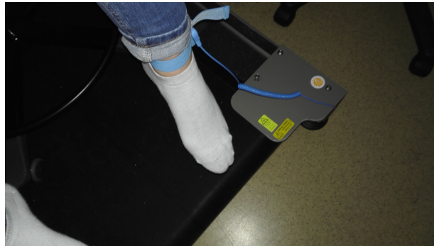
Figure 30.: An ankle strap was used in order to ground the participant, hence reducing interference with the recorded EEG data.
