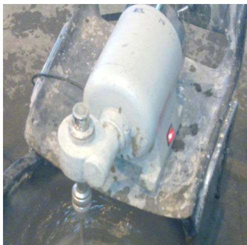
Figure 4.3 Mixer used for the mixing of the drilling fluid
