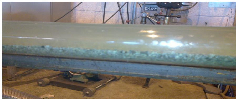
Figure 4.8: Erosion of cuttings at with water flow in 15 cm washout
