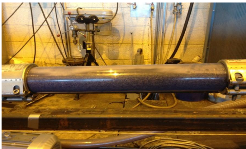
Figure 4.6: Erosion of cuttings with water flow in 15 cm washout
