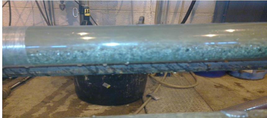
Figure 4.7: Erosion of cuttings with water flow in 15 cm washout
