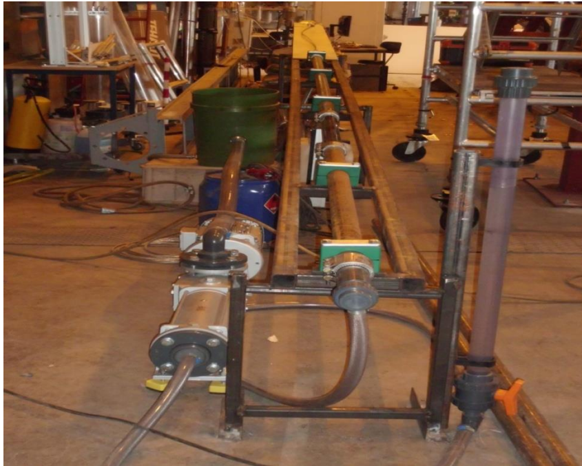
Figure B5: The flow loop setup
