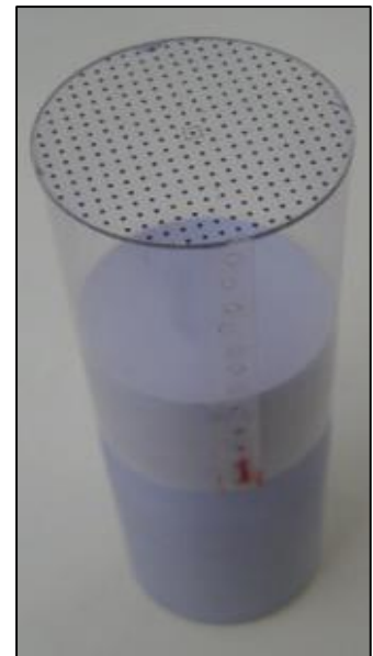
Figure 19: A calibration grid and its bracket made by Doorne & Hendrik (2004).
