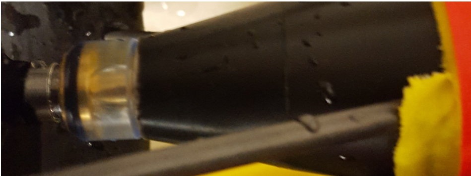
Figure 6.2: Cartridge seal: Air bubble "full" in the starboard thruster
