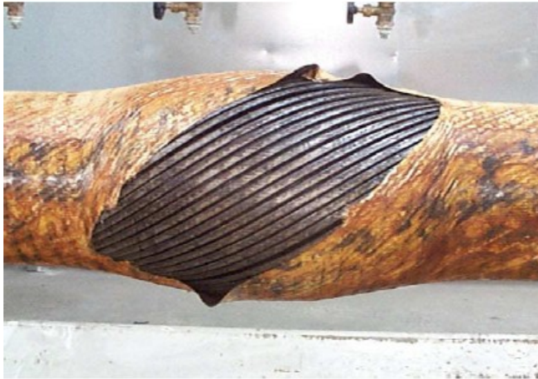
Figure 2.4: Radial buckling behavior (Østergaard et al. [15])
