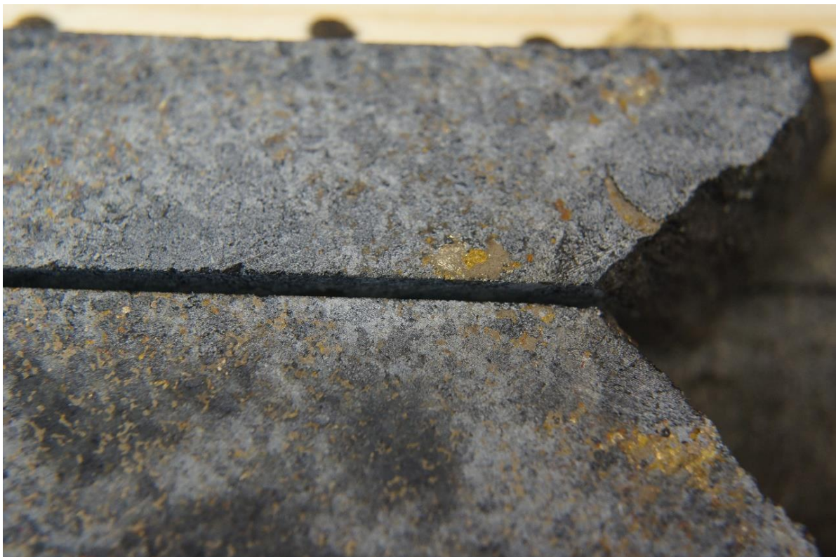
Figure 6.4: Split drill core from RF-1, showing the sulfide enrichment in the Cu-Ni reef.
