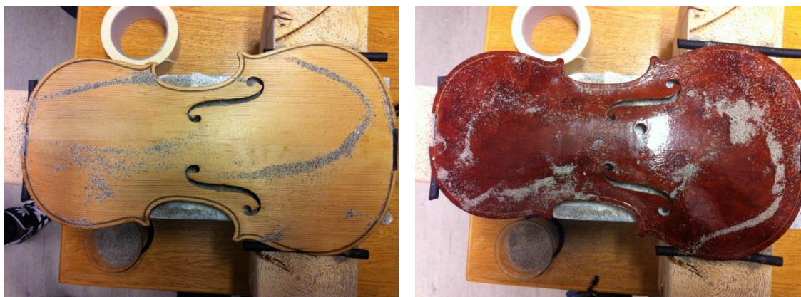
Figure 5: Left: Stradivari-copy top plate with node lines at 570 Hz. Right: Hagetrø preformed plywood top plate with similar node lines at 740 Hz. (From [5])
